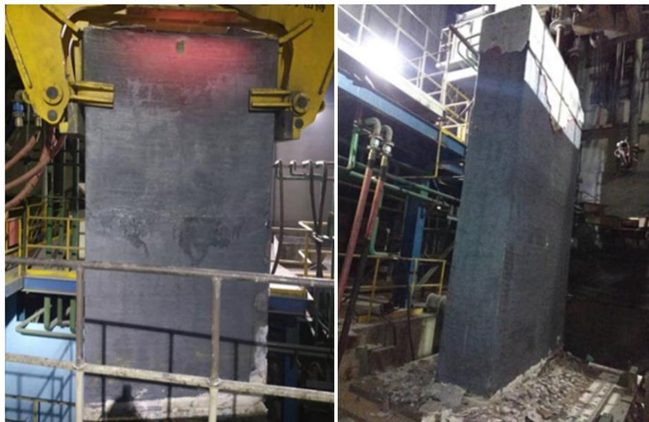
**Figure 16.** Electroslag ingots with a dimension of 620 mm × 2060 mm × 3630 mm produced after the improved process.
