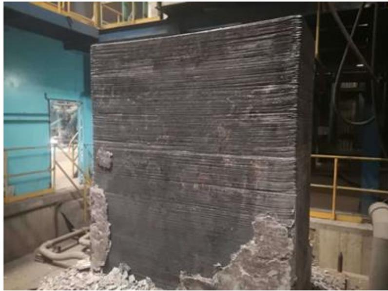
**Figure 15.** Electroslag ingots with a dimension of 620 mm × 2060 mm × 3630 mm produced before the improved process.
