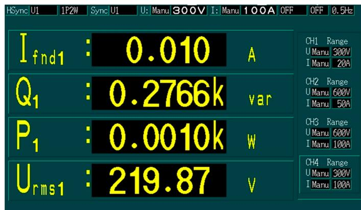
Figure 27. Parameters after load resonance.
