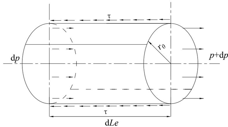
**Figure 2.** Flow diagrammatic sketch of Newtonian fluid in the pores of porous media.
