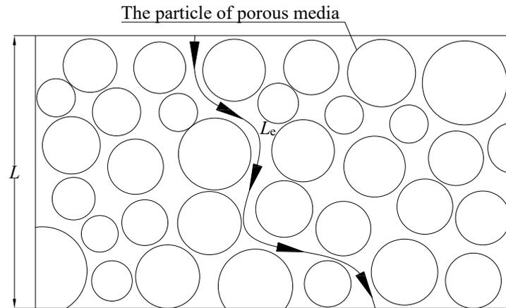
**Figure 1.** Diagrammatic sketch of fluid's flow paths in porous media.
