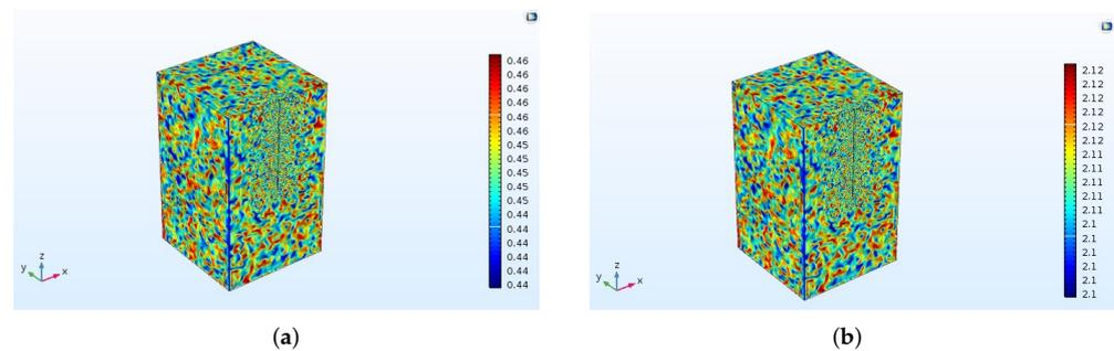
**Figure 6.** The simulation results of porosity and permeability coefficient distribution of gravel soil with particle gradation of 3~5 mm: (a) porosity distribution; (b) permeability coefficient distribution.
