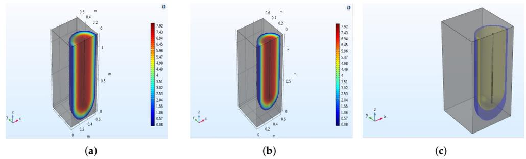
**Figure 7.** Numerical simulation results of the column-hemispherical penetration diffusion of Newtonian cement slurry in gravel soil; (a) The results without considering the tortuosity effect; (b) the results considering the tortuosity effect; (c) the comparison of the two results.
