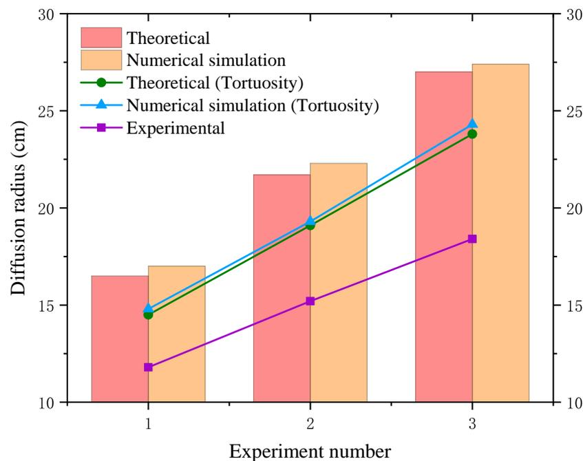
**Figure 8.** Comparison of theoretically calculated, numerically simulated, and experimental values of the hemispherical diffusion radius.
