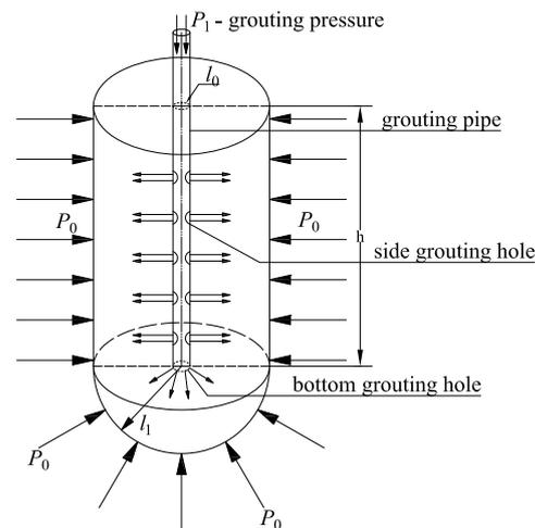
**Figure 3.** Column-hemispherical penetration diffusion model of Newtonian fluid in porous media.
