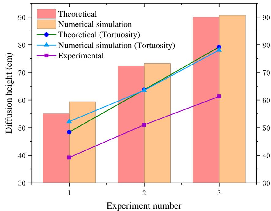
**Figure 9.** Comparison of theoretically calculated, numerically simulated, and experimental values of the column diffusion height.
