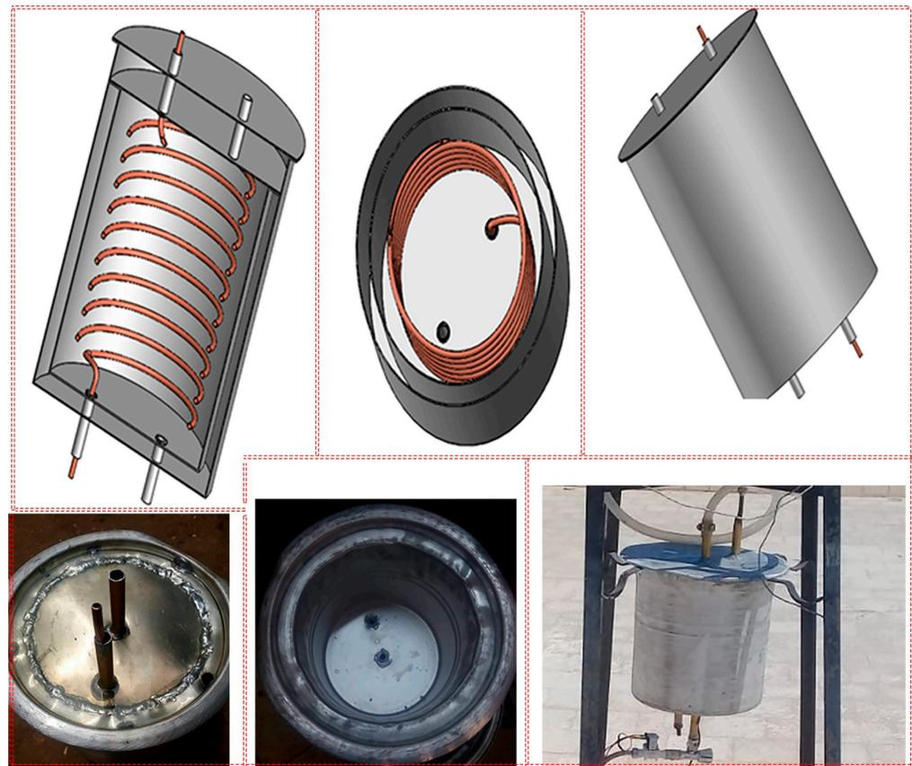
**Figure 5.** Different details of the condenser investigated.
