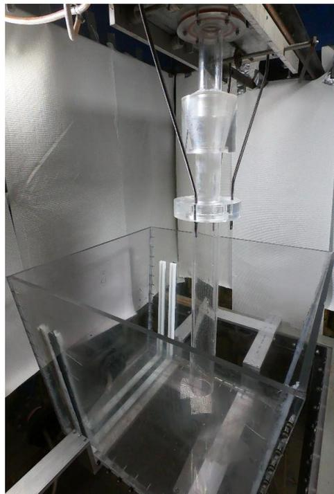
**Figure 7.** Experimental set-up with water model Ladle Shroud and tundish tank.
