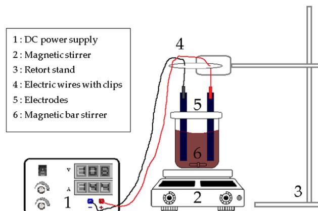
**Figure 1.** Electrochemical oxidation pre-treatment set-up.
