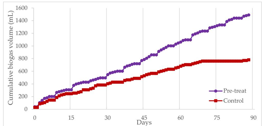
**Figure 6.** Cumulative biogas production of control and pre-treated digesters.
