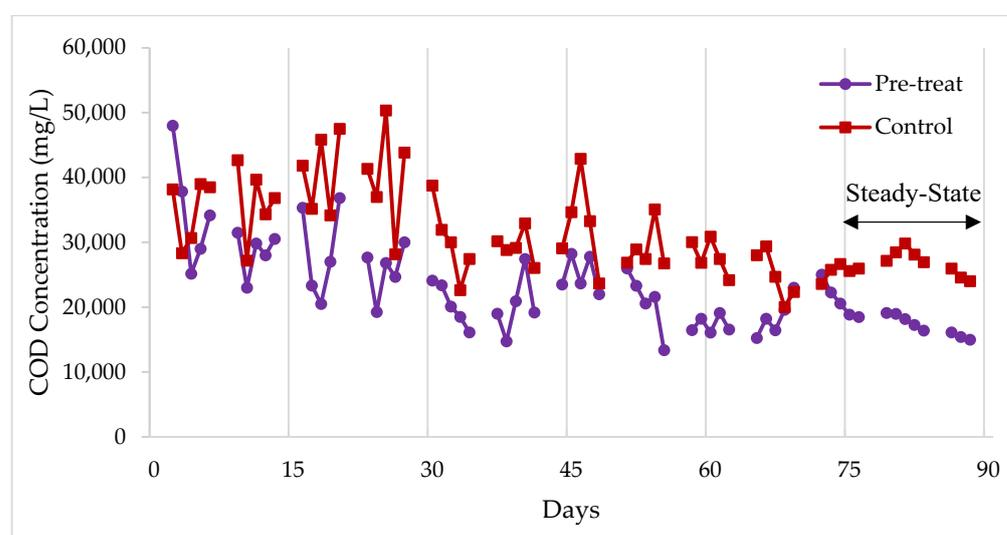
**Figure 5.** Concentration of COD between the control and pre-treated digesters.
