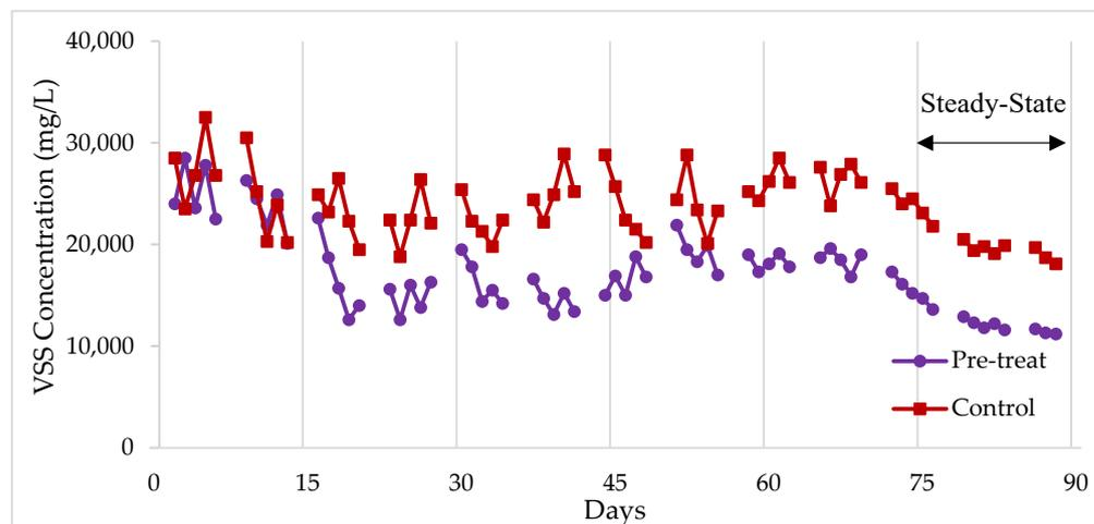
**Figure 4.** Concentration of VSS between control and pre-treated digesters.
