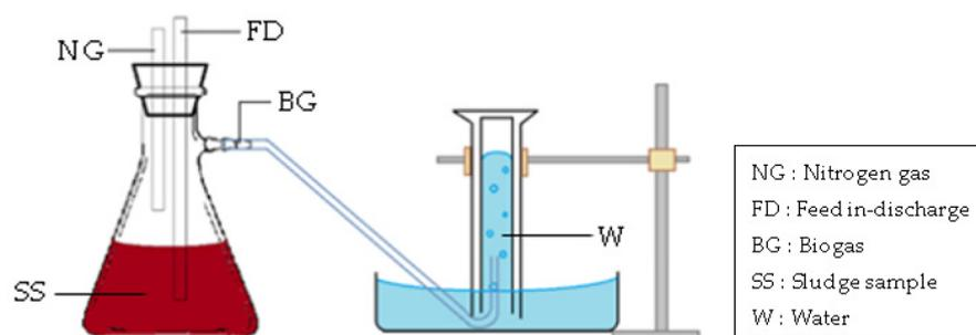
**Figure 2.** Anaerobic digester set-up.
