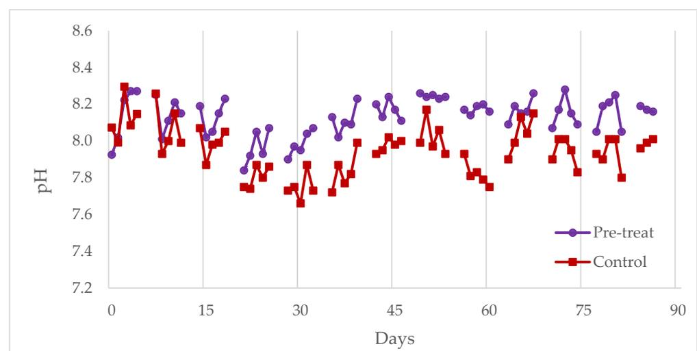
Figure 3. pH variation of control and pre-treated digesters.
