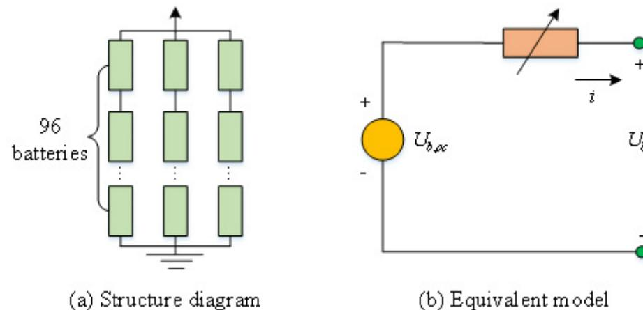
**Figure 2.** Equivalent Model and Structure Diagram of the Power Battery Pack.
