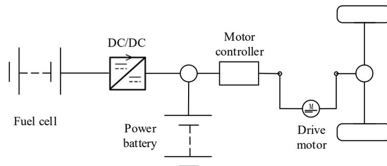
**Figure 1.** Power System Structure of a FCEV.
