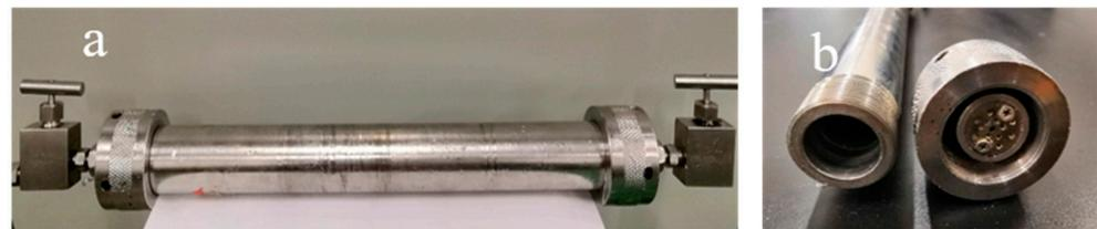
Figure 1. One-dimensional sandpack: (a) lateral view, (b) end view.
