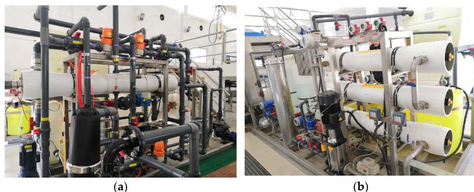
**Figure 2.** On-site pictures of UF and NF. (a) UF unit; (b) NF unit.
