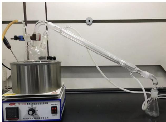
**Figure 2.** The experimental device of the chlorination reaction.
