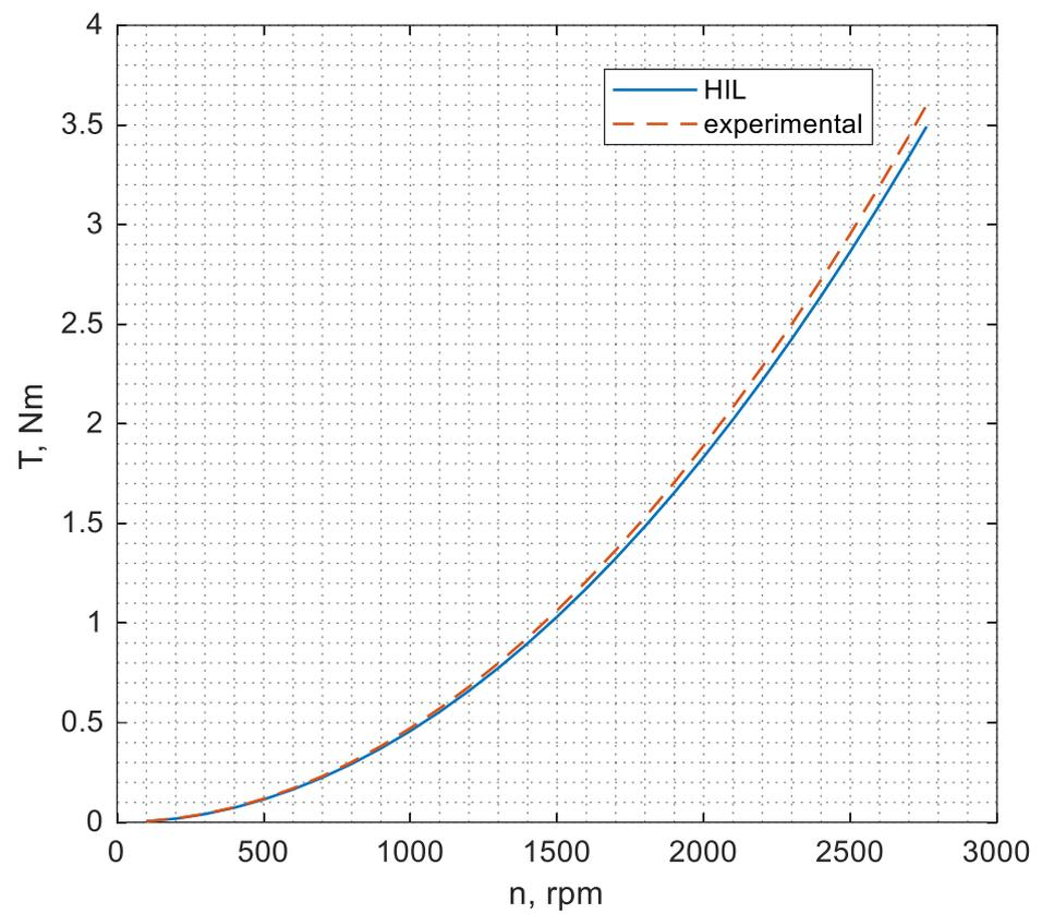
Figure 5. Torque–speed ( $T$ – $n$ ) characteristics of the simulated and real pumps.
