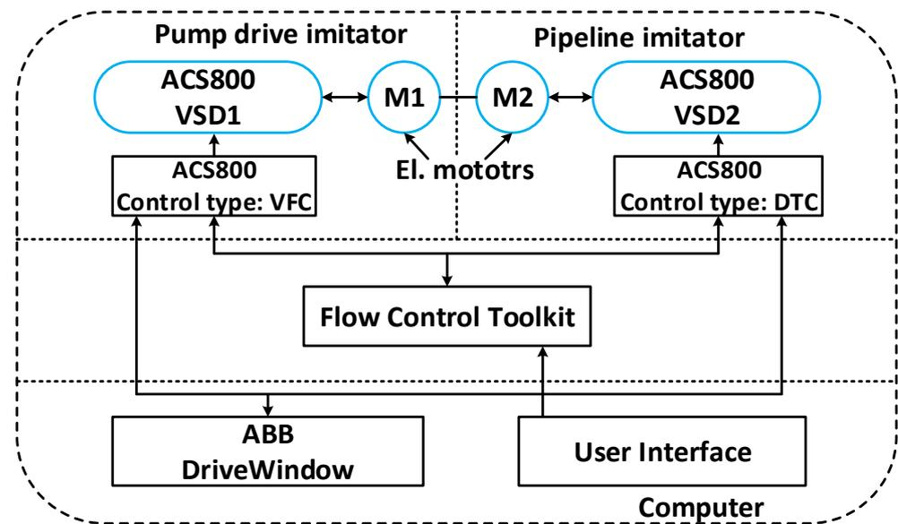
Figure 2. HIL centrifugal pump and pipeline imitators.
