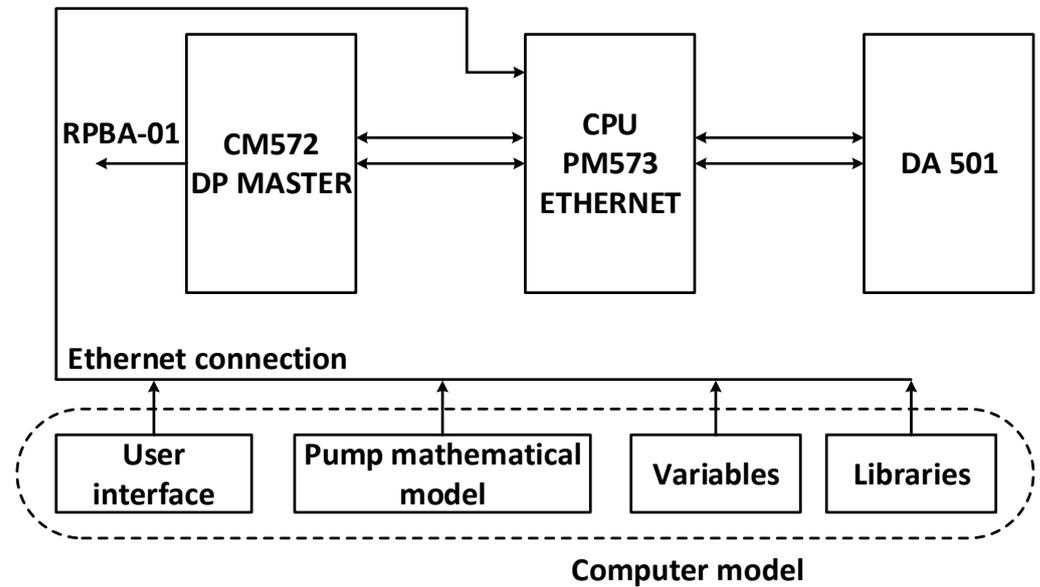
Figure 3. AC500 PLC structure.
