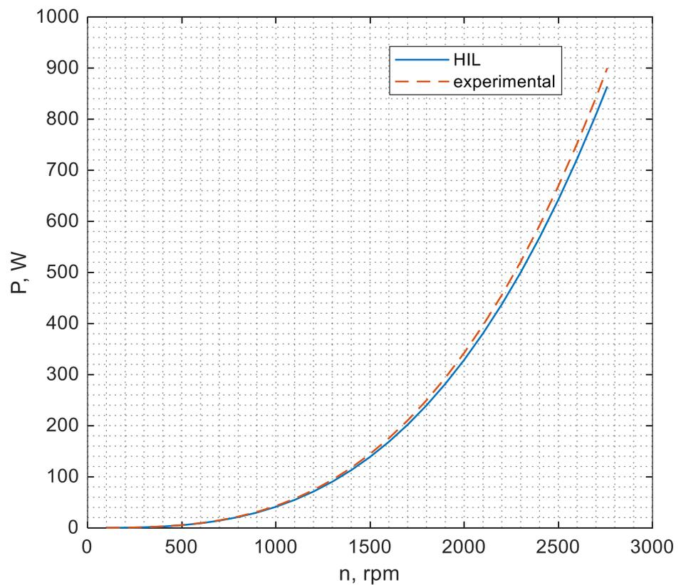
Figure 6. Power–speed ( $P$ – $n$ ) characteristics of the simulated and real pumps.
