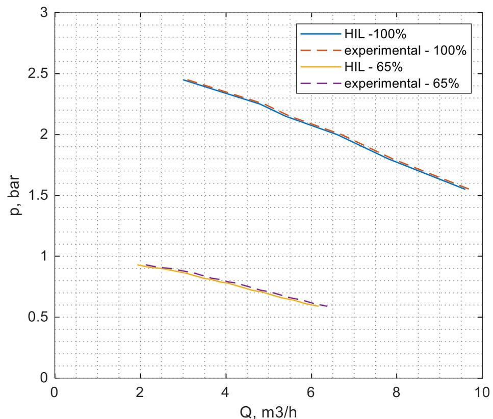
**Figure 7.** Flow–pressure ( $p$ – $Q$ ) characteristic of the simulated and real pumps at rated and 65% of the rated speed.
