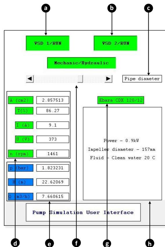
Figure 4. Software developed to control HIL test-bench.
