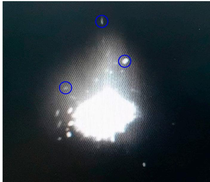
**Figure 2.** Phenomenon of the charge being blown up by the gas flow at the center of the furnace throat.
