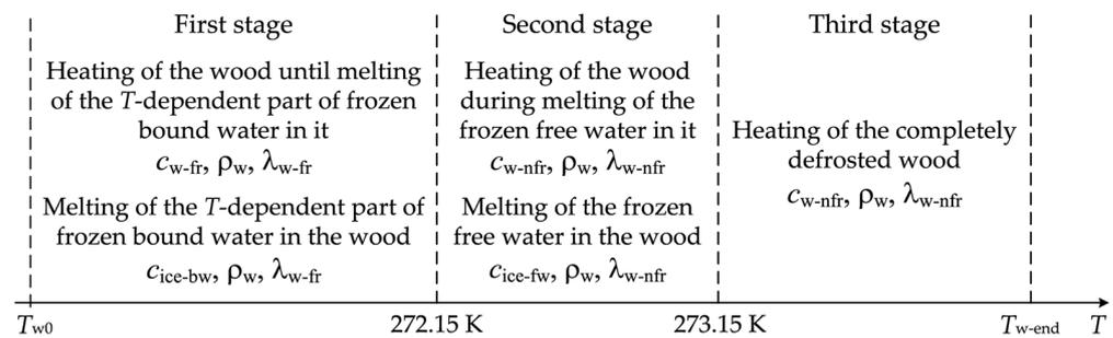
**Figure 1.** Stages of the wood defrosting process and thermo-physical characteristics of wood used in them.
