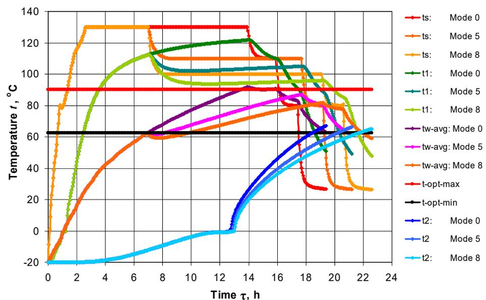
**Figure 3.** Changes in  $t_s$ ,  $t_{w\text{-avg}}$ ,  $t_1$ , and  $t_2$  of the prisms during steaming Mode 0, Mode 5, and Mode 8, depending on  $\tau$ .
