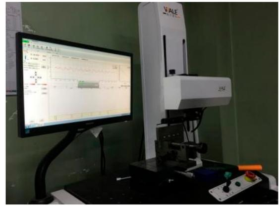
(b) Contact measuring instrument RC50H
