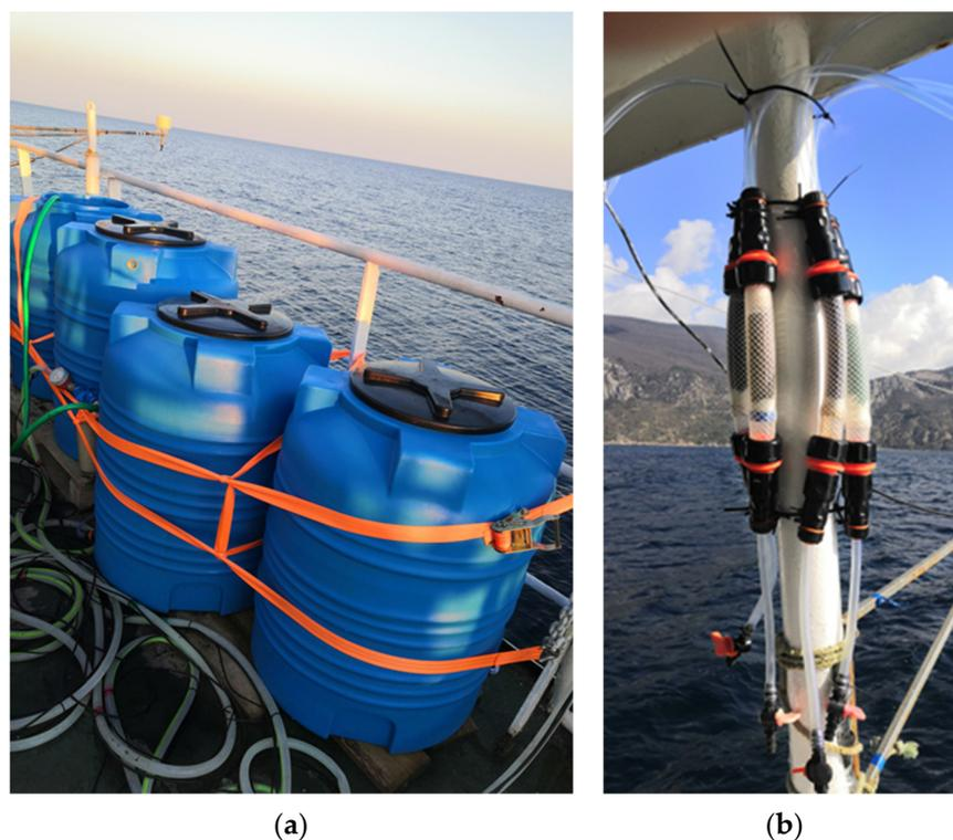
**Figure 1.** Sorption of  $^{137}\text{Cs}$  from seawater: (a) sampling barrels; (b) columns with sorbents.
