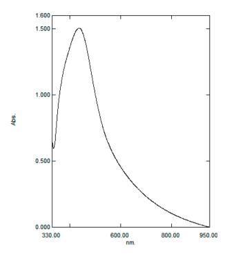
**Figure 1.** UV-vis absorbance spectra of AgNPs prepared with aqueous *A.nilotica* pod extract.
