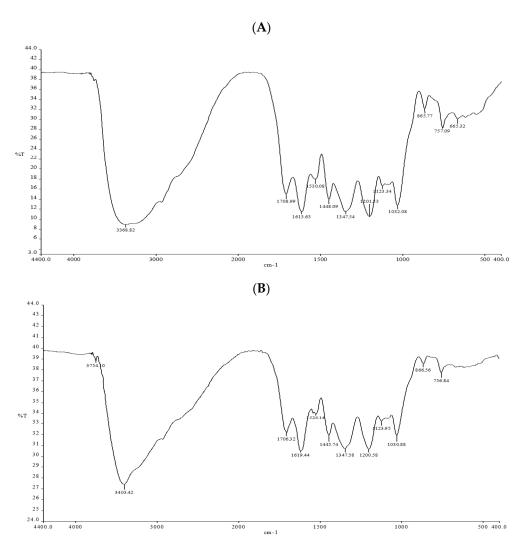
**Figure 6.** FTIR of **(A)**. Aqueous *A. nilotica* pod extract, **(B)** Biosynthesized AgNPs prepared with aqueous extract of *A. nilotica* pods.
