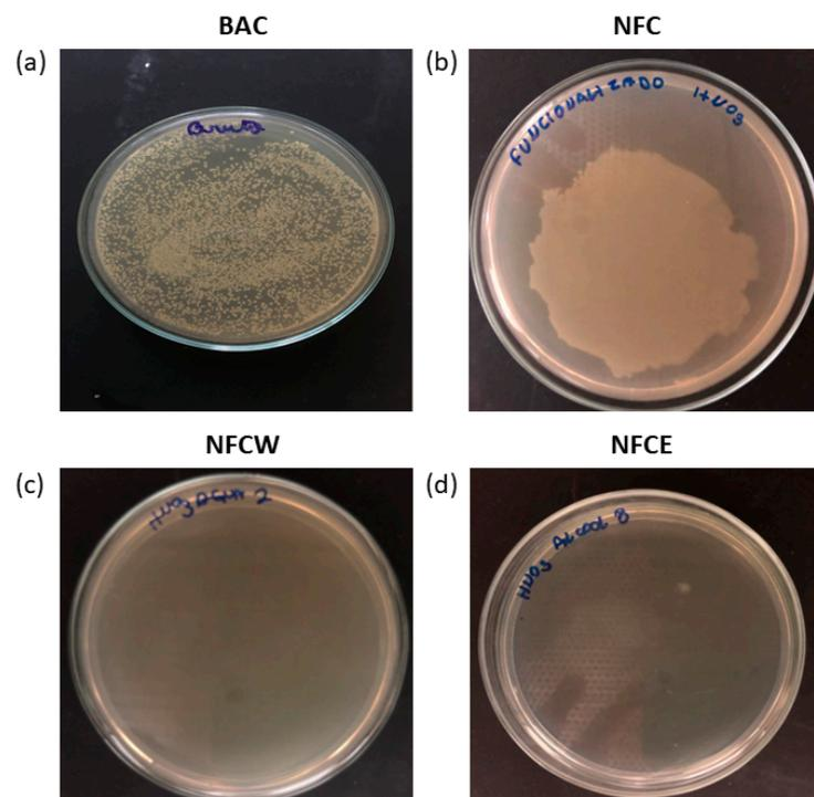
**Figure 4.** Microbiological test images of activated carbon samples (a) BAC—Babassu Activated Carbon, (b) NFC—Nitric Functionalized Carbon, (c) NFCW—Nitric Functionalized Carbon impregnated with Water extract, (d) NFCE—Nitric Functionalized Carbon impregnated with Ethanol extract).
