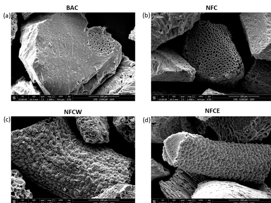
**Figure 1.** SEM images of activated carbon samples (a) BAC—Babassu Activated Carbon, (b) NFC—Nitric Functionalized Carbon, (c) NFCW—Nitric Functionalized Carbon impregnated with Water extract, (d) NFCE—Nitric Functionalized Carbon impregnated with Ethanol extract) at 1000× magnification.
