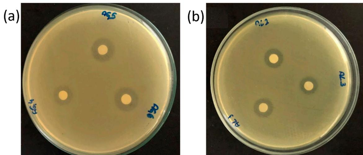
**Figure 3.** Antimicrobial susceptibility testing by disc diffusion for (a) water-based garlic extract,  $16 \pm 1.3$  mm, and (b) ethanol-based garlic extract,  $14 \pm 1.0$  mm (mean and standard deviation values obtained from 10 replicates).
