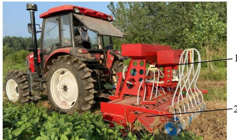
**Figure 6.** Field test of FA: 1—spiral cone centrifugal FA; 2—2BYQ-8 rapeseed seeder.
