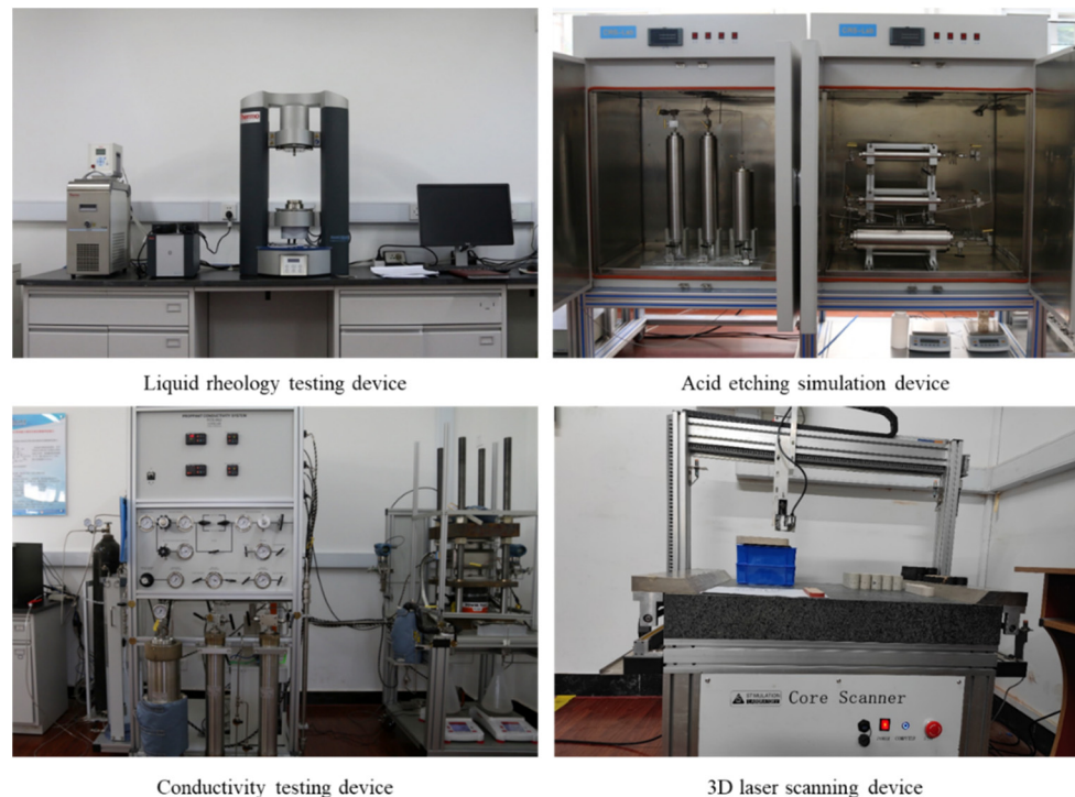
Figure 2. Acid fracturing conductivity test system.
