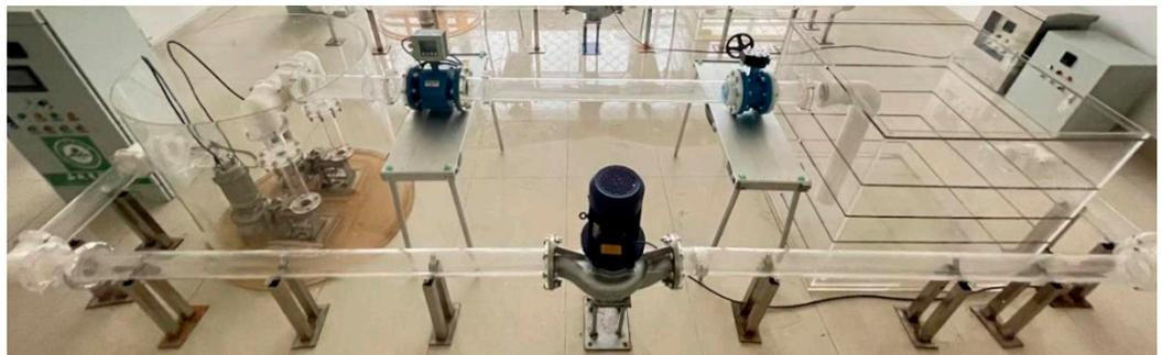
**Figure 5.** Physical diagram of centrifugal prefabricated pumping station test bench.
