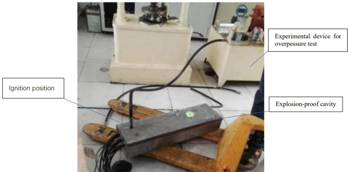
**Figure 20.** Testing setup of pressure test.
