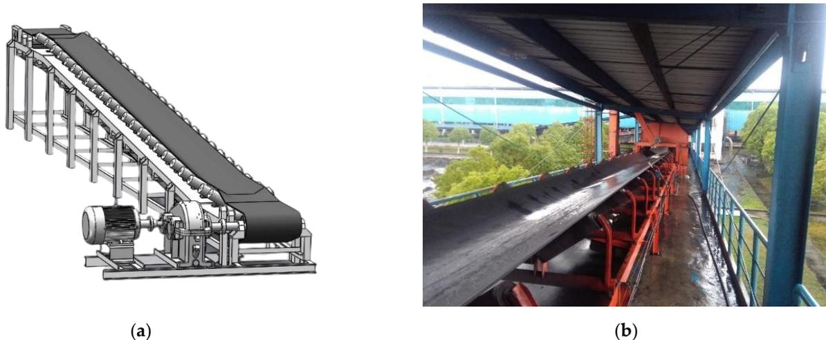
**Figure 1.** Coal mine belt conveyor: (a) illustration of model; (b) object pictures.
