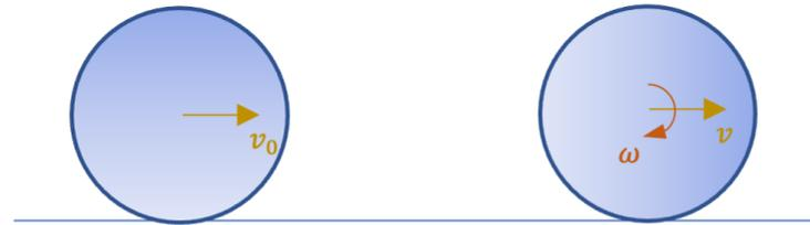
**Figure A1.** Particle sliding on a wall with initial velocity  $v_0$ . Due to attrition, the translational energy is progressively converted into rotational energy.
