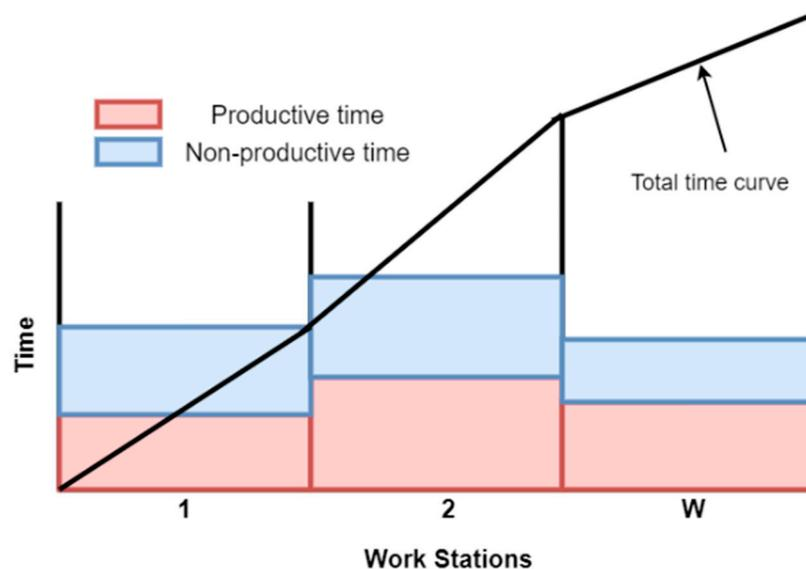
Figure 3. Representation of time components of different workstations.
