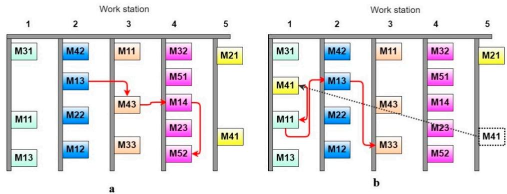
Figure 14. Production stage designs for the balancing problem of case study 1. (a) First configuration design, (b) second configuration design.
