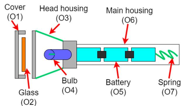
Figure 12. A hand light and its sub-assemblies adapted from [8,52] (case study 2).
