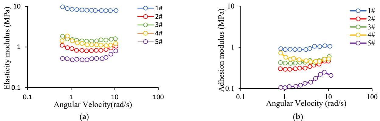
**Figure 2.** Rheological measurement results. (a) The relationship between elastic modulus and angular velocity. (b) The relationship between viscous modulus and angular velocity.
