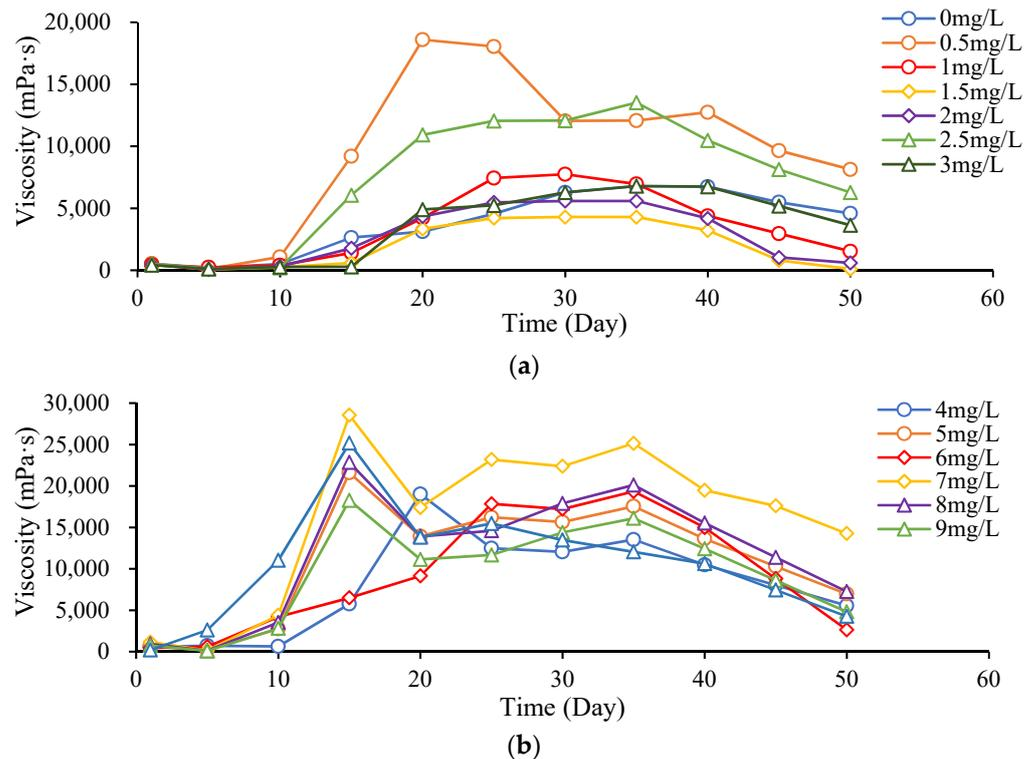
**Figure 3.** Effect of dissolved oxygen content on the gel strength of weak gels. (a) 0–3 mg/L Dissolved oxygen content. (b) 4–10 mg/L Dissolved oxygen content.
