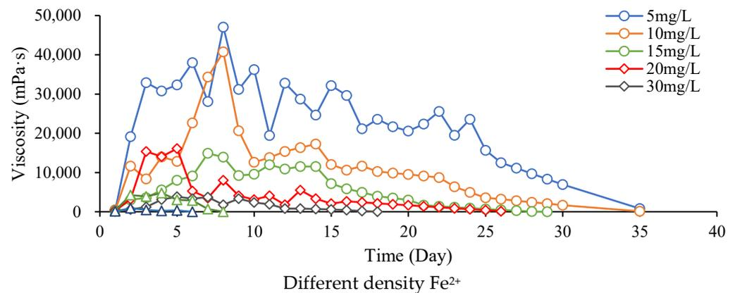
**Figure 6.** Effects of  $\text{Fe}^{2+}$  and  $\text{Fe}^{3+}$  on the gel-forming properties of weak gels.
