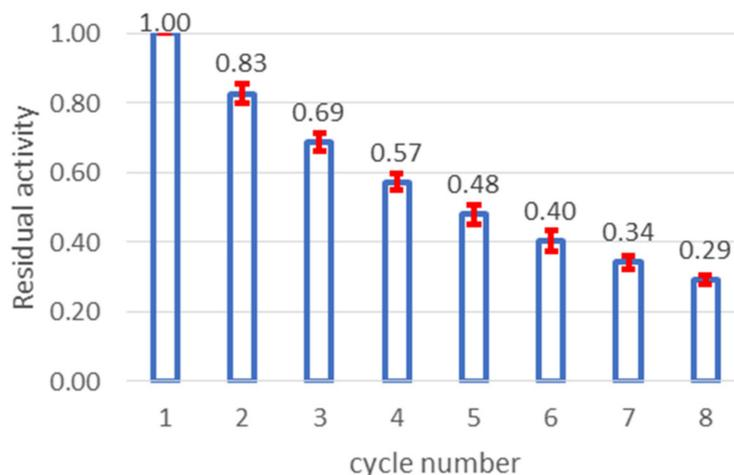
**Figure 6.** Residual activity evolution for several consecutive hydrolysis cycles. Conditions: 20 g/L (58.5 mM) cellobiose in 100 mM citrate buffer pH 5.0 under orbital shaking at 400 rpm and 50 °C.
