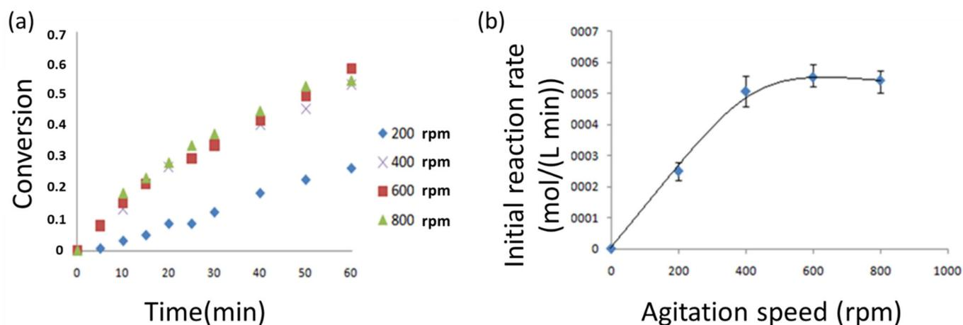
**Figure 3.** Effect of stirring speed on hydrolysis of cellobiose catalyzed by immobilized  $\beta$ -glucosidase (ASA-1000) at various reactor stirring speeds. Reaction conditions: 100 mg of immobilized RN8 derivative; temperature 40 °C; 2 mL sodium citrate buffer 100 mM pH 5.0; 20 g/L cellobiose. (a) Progress curves and (b) Initial observed rate versus agitation speed.
