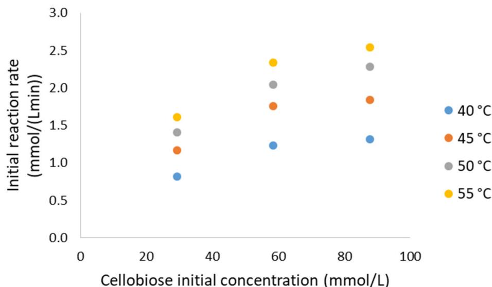
**Figure 4.** Initial reaction rate versus initial concentration of cellobiose at several temperatures.
