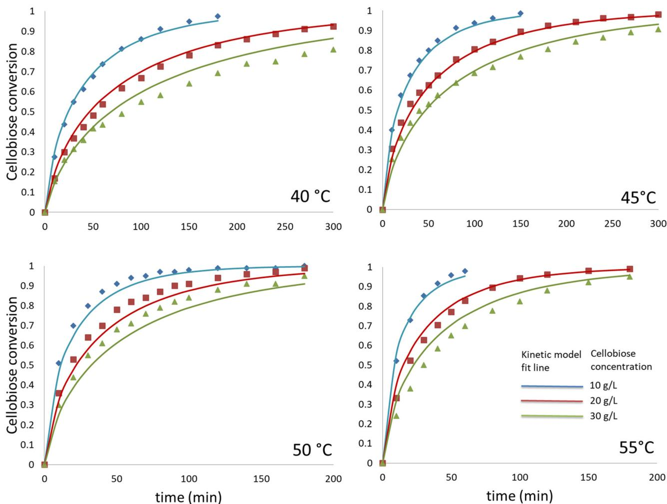
**Figure 5.** Fit of the proposed model (in lines) to data retrieved at all temperatures (points) tested and several cellobiose initial concentrations. Other reaction conditions: 100 mg of immobilized RN8 derivative; 2 mL sodium citrate buffer 100 mM pH 5.0.
