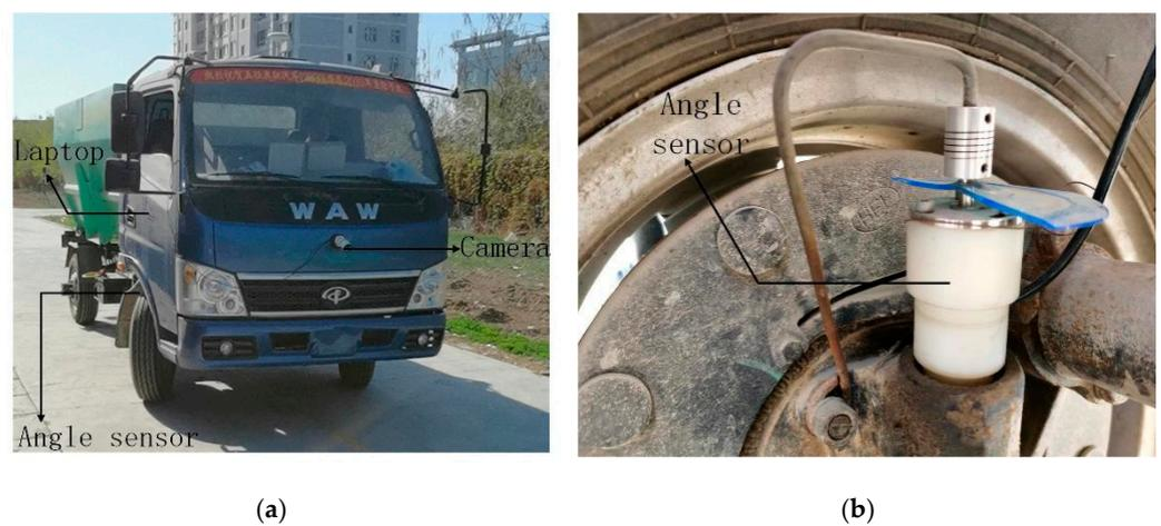
Figure 10. Equipment layout. (a) Fixed position of equipment. (b) Position of angle sensor.
