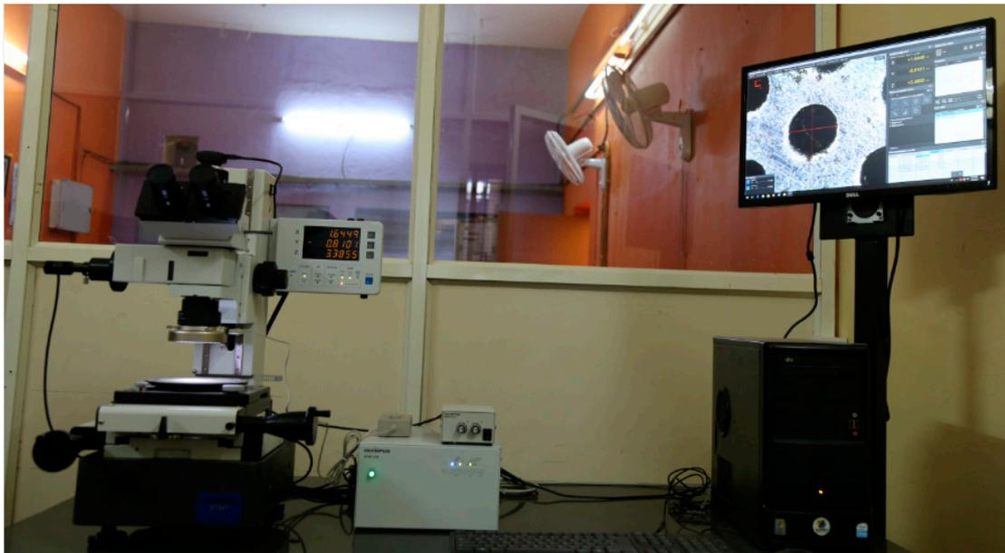
**Figure 5.** Light microscope used for hole quality assessment.
