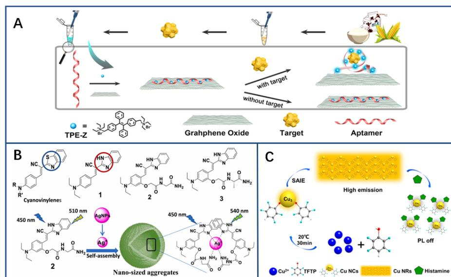
**Figure 7.** (A) The scheme of the label-free fluorescence aptasensor for AFB<sub>1</sub> detection based on TPE-Z/AFB<sub>1</sub> aptamer/GO [104]; (B) the assembling mode of fluorophore with Ag<sup>+</sup> [106]; (C) the mechanism of Cu NCs in histamine detection [107].
