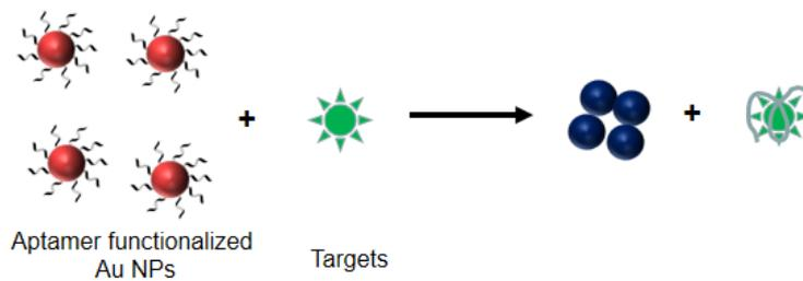
**Figure 4.** Several schemes of colorimetric sensors based on Au NPs' aggregation.
