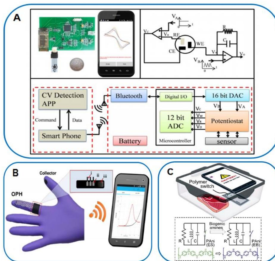
**Figure 18.** (A) An electrochemical detections sensor based on combination of screen-printed electrodes and smartphone [201]; (B) a wearable and disposable electrochemical platform based on a combination of a nitrile experimental glove surface and smartphone [202]; (C) switchable NFC technology for the detection of food spoilage with smartphone [205].
