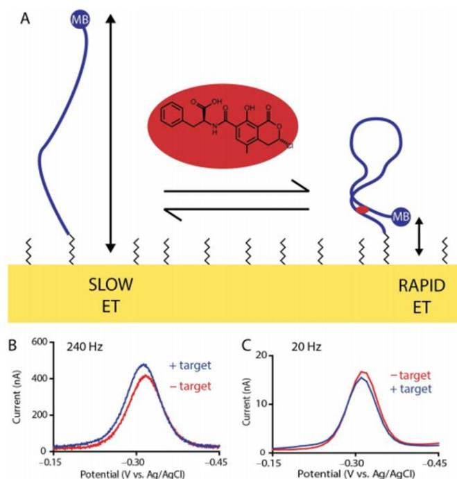
**Figure 10.** The scheme of electrochemical aptasensors for monitoring OTA. The sensing interface consists of methylene blue-modified DNA aptamers (A), and sensor current changes are observed at higher (B) and lower (C) square wave frequencies [133].
