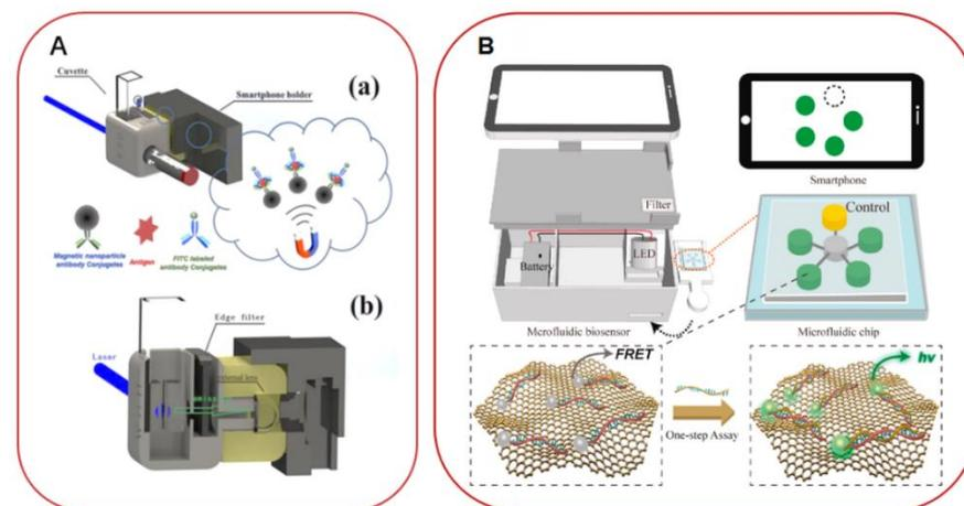
**Figure 17.** (A) Schematic diagram (a) and profile (b) of a smartphone-based fluorescence biosensors for *E. coli* O<sub>157</sub>:H<sub>7</sub> detection [191]; (B) smart biosensor for simultaneous detection of multiplex foodborne bacterial ssDNA [196].
