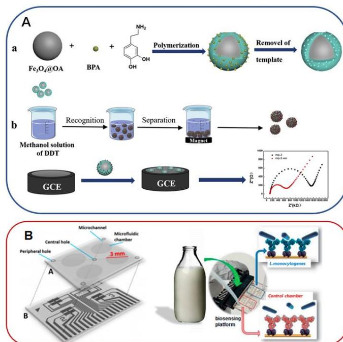
**Figure 9.** (A) Electrochemical impedance sensor scheme for detecting DDT by EIS, including synthesis of PDA@Fe<sub>3</sub>O<sub>4</sub> MIP MNPs (a) and sensor construction (b); (B) four microelectrode array modes (A) and platform assembly mode (B) of sensing modules in a label-free miniaturized platform protocol for the detection of *L. monocytogenes* by EIS [132].
