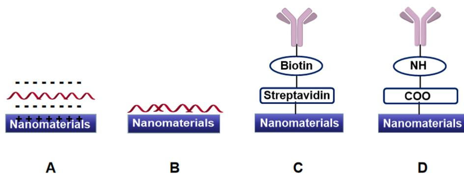
**Figure 3.** The scheme for the combination of nanomaterials and bioreceptors of recognition element, including electrostatic interaction (A),  $\pi$ - $\pi$  stacking (B), biomolecular links (C), classic amide coupling reactions (D).
