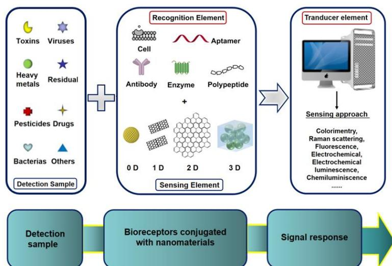
**Figure 2.** Schematic of nanomaterial-based sensor and biosensor construction.
