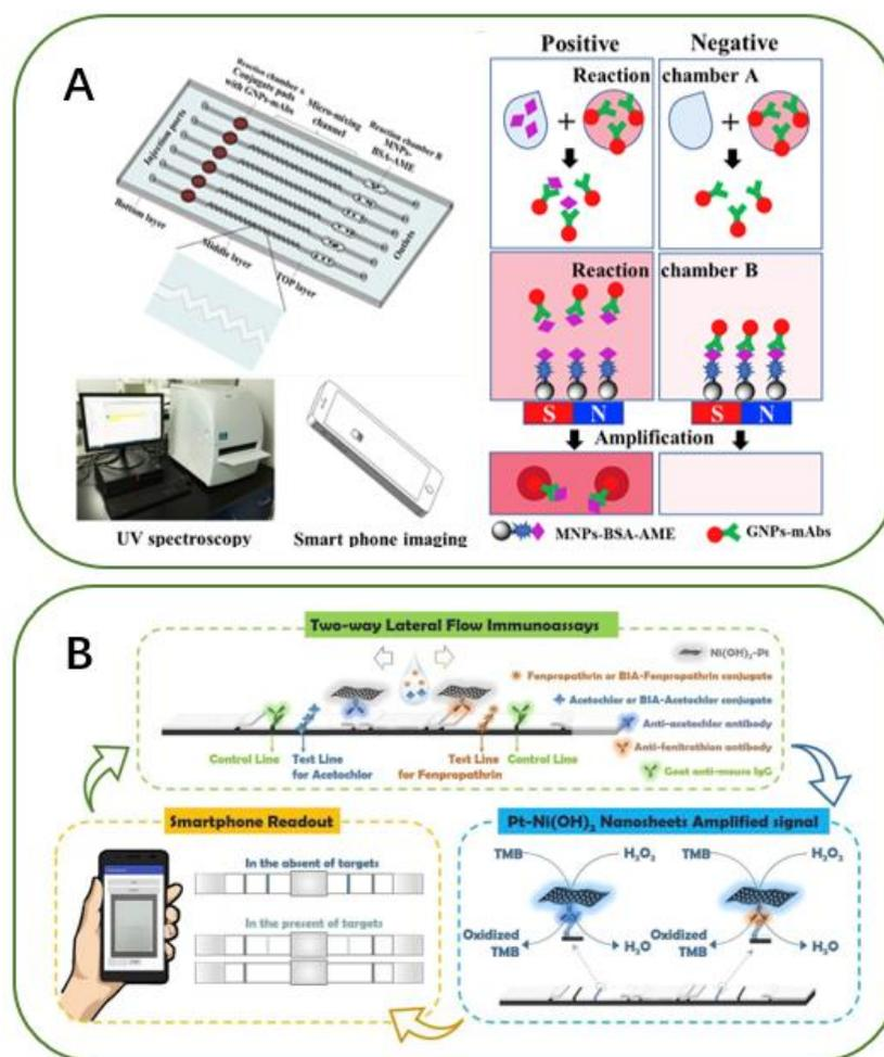
**Figure 15.** (A) Schematic diagram of a microfluidic colorimetric immunoassay device based on Au NPs [181]; (B) schematic diagram of bidirectional lateral flow immunoassay equipment based on NSs amplification [182].
