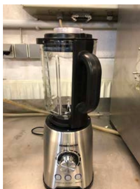
Figure S1. MX 1250, Rommelsbacher: A high shear blender equipped with a rotor and six blades used to produce dry water. The Maximum speed is 22,000 \text{ min}^{-1} and the blade diameter is approximately 0.07 m.
