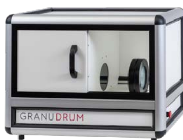
Figure S3. GranuDrum by GranuTools: A device to measure the dynamic angle of repose based on the rotating drum method. The black cylinder was filled to 50 % by volume and speeds were varied between 2 \text{ min}^{-1} and 50 \text{ min}^{-1} . Note, the glass screens were replaced with Perspex discs to avoid problems during measurements (water spreading on the screen). Image source: https://www.granutools.com/en/granudrum
