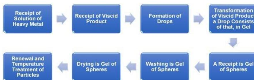
**Figure 1.** Sol–gel-process steps for producing  $\text{Al}_2\text{O}_3$  granules.
