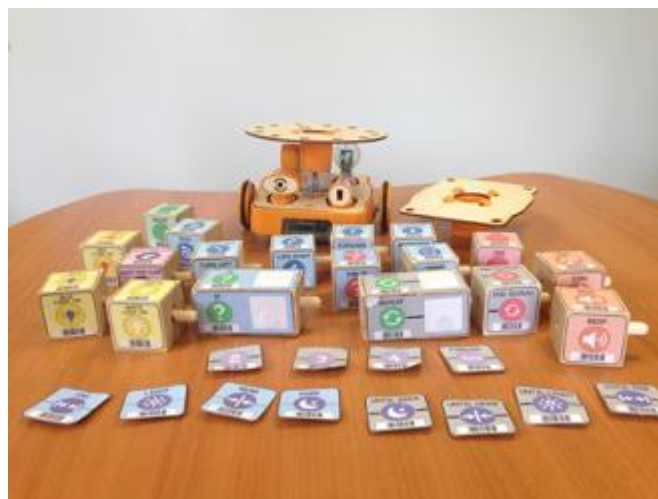
Figure 3. Blocks for programming KIBO and a sample KIBO program. This program tells the robot to spin, shake, move backward, move forward, and turn a red light on.
