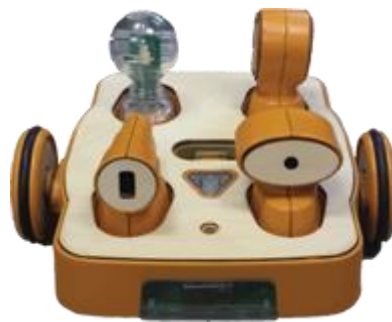
Figure 2. KIBO robot with sensors and light output attached.
