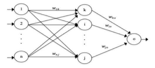
Figure 2. Architecture of the feed-forward neural network.
