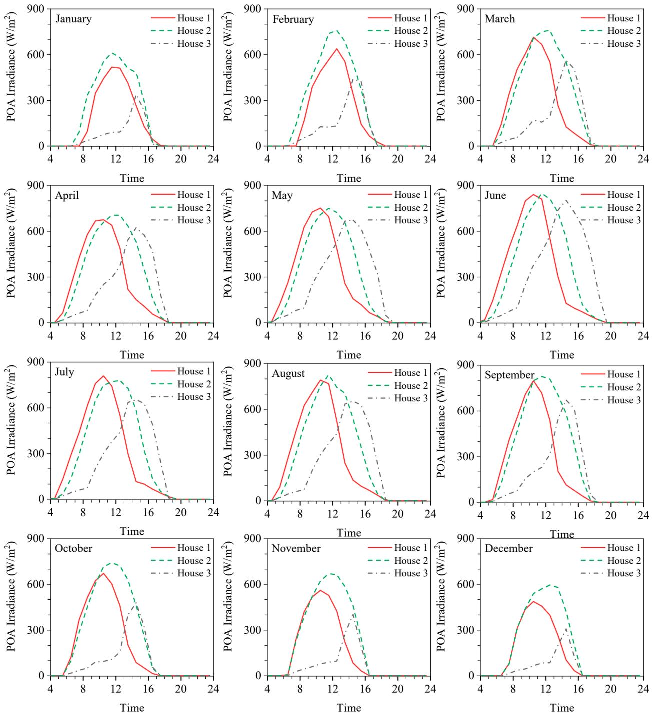
**Figure 3.** Simulated POA irradiance data for the CSP case study.
