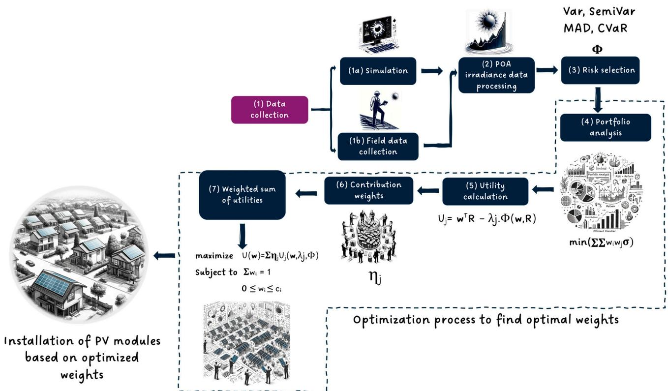
Figure 1. A step-by-step methodology for designing a portfolio-based community solar project.
