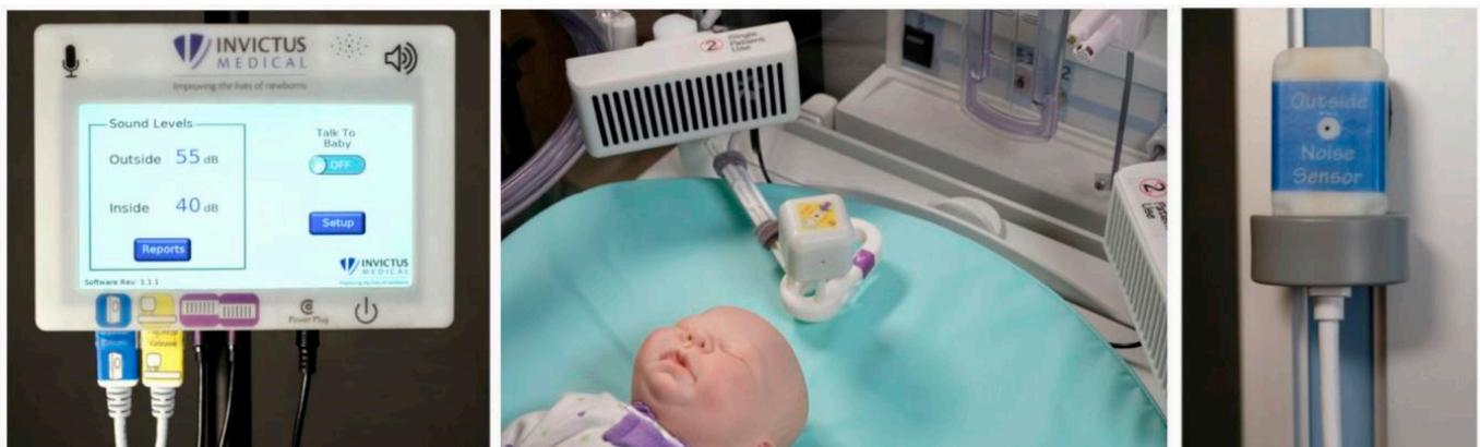
**Figure 1.** Neoasis™ system: on the left is the control unit with the external noise sensor, in the center are the speakers and the internal noise sensor, on the right is the additional “outside” noise sensor. <http://www.invictusmed.com/neoasis/> (accessed on 6 February 2021).
