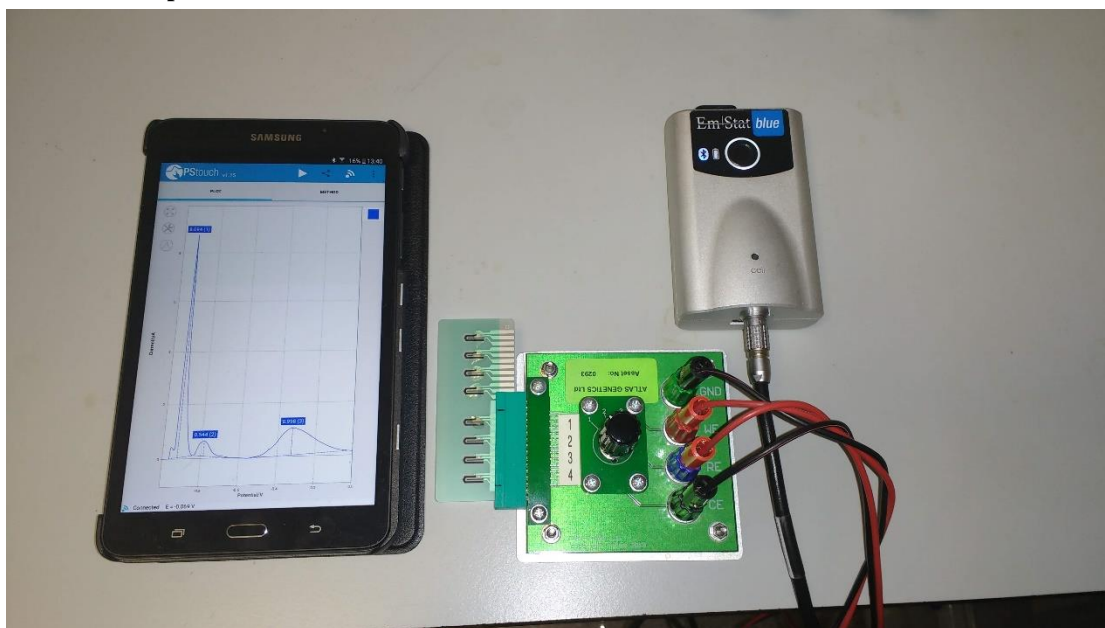
Figure S6 – Photograph of handheld potentiostat setup. PalmSens EmStat 3 Blue potentiostat (right) connected to electrode rig (middle), and via Bluetooth to a tablet (left) running PS Touch.
