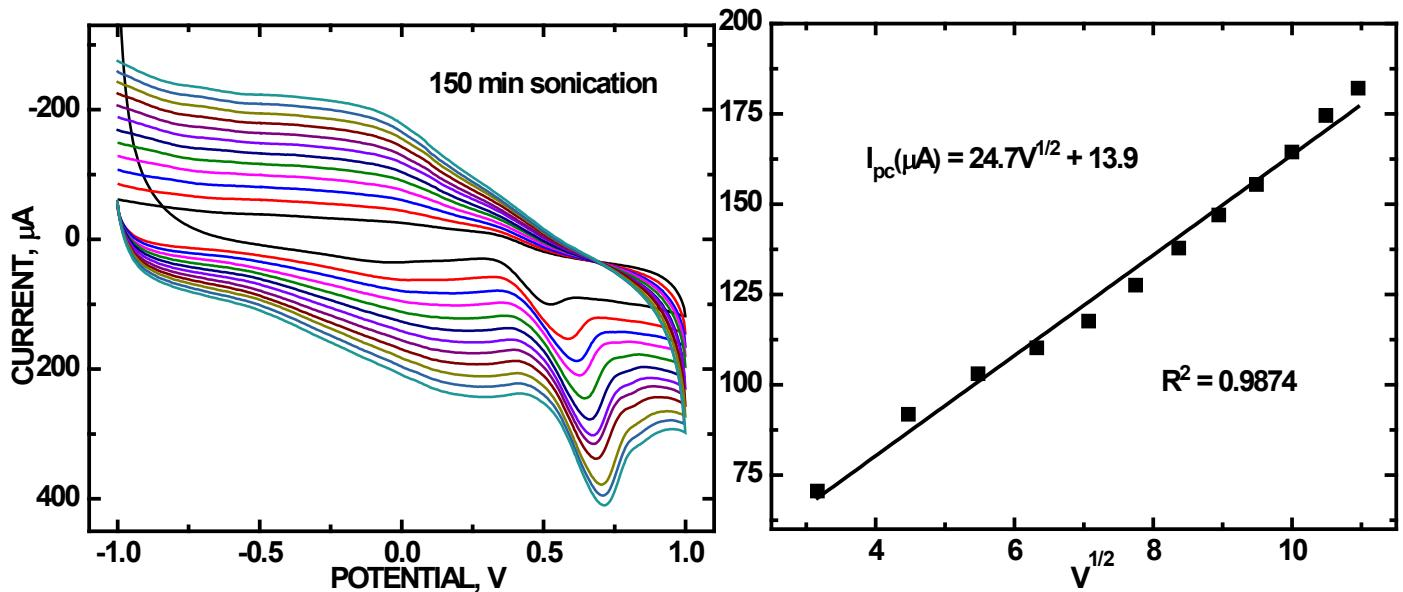
**Figure S5.** CVs of 10 mM UA in PBS (pH = 7.0) at scan rates between 10-100 mV·s<sup>-1</sup> for a 150 min refluxed ZnO/COOH-MWNT composite (left panel). Linear least squares plot from Randles-Sevcik analysis (right panel).
