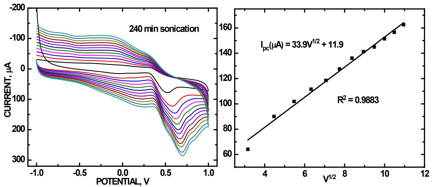
**Figure S8.** CVs of 10 mM UA in PBS (pH = 7.0) at scan rates between  $10\text{-}100 \text{ mV}\cdot\text{s}^{-1}$  for a 240 min refluxed ZnO/COOH-MWNT composite (left panel). Linear least squares plot from Randles-Sevcik analysis (right panel).
