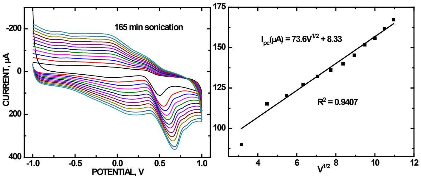
**Figure S6.** CVs of 10 mM UA in PBS (pH = 7.0) at scan rates between 10-100 mV·s<sup>-1</sup> for a 165 min refluxed ZnO/COOH-MWNT composite (left panel). Linear least squares plot from Randles-Sevcik analysis (right panel).
