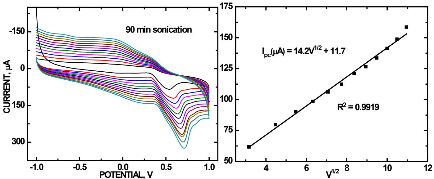
**Figure S3.** CVs of 10 mM UA in PBS (pH = 7.0) at scan rates between 10-100 mV·s<sup>-1</sup> for a 90 min refluxed ZnO/COOH-MWNT composite (left panel). Linear least squares plot from Randles-Sevcik analysis (right panel).
