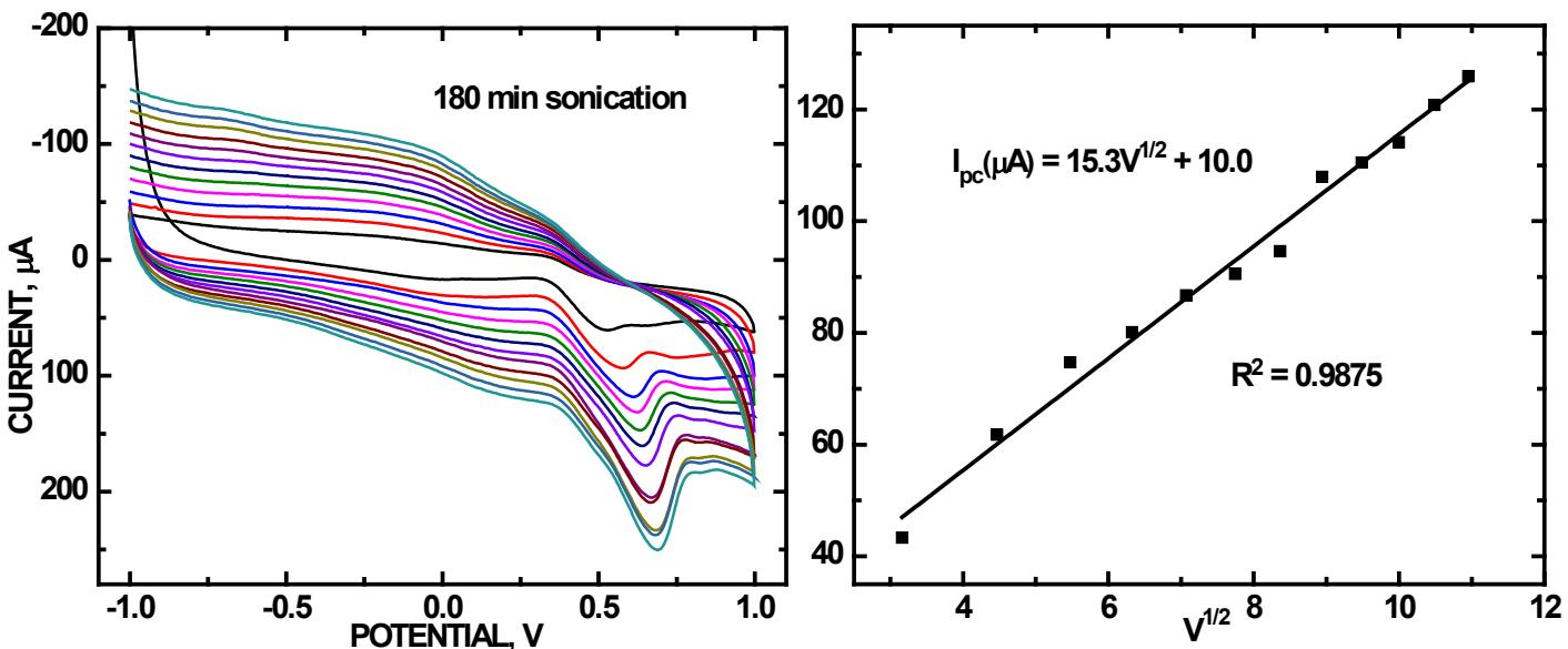
**Figure S7.** CVs of 10 mM UA in PBS (pH = 7.0) at scan rates between 10-100 mV·s<sup>-1</sup> for a 180 min refluxed ZnO/COOH-MWNT composite (left panel). Linear least squares plot from Randles-Sevcik analysis (right panel).
