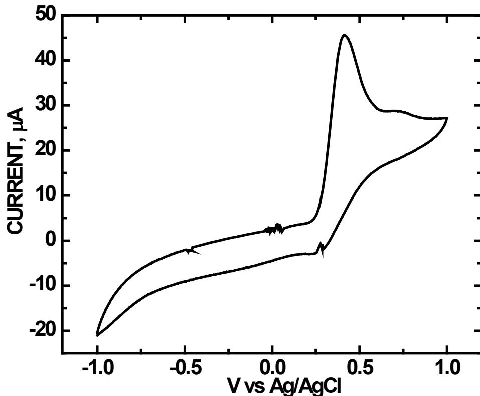
**Figure S1.** CV of 10 mM UA in PBS ( $\text{pH} = 7.0$ ) at scan rates between  $50 \text{ mV}\cdot\text{s}^{-1}$  using only refluxed ZnO NPs.
