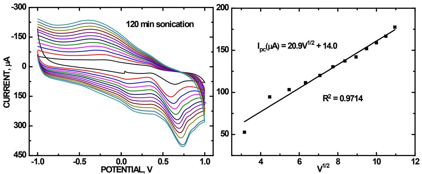
**Figure S4.** CVs of 10 mM UA in PBS (pH = 7.0) at scan rates between 10-100 mV·s<sup>-1</sup> for a 120 min refluxed ZnO/COOH-MWNT composite (left panel). Linear least squares plot from Randles-Sevcik analysis (right panel).
