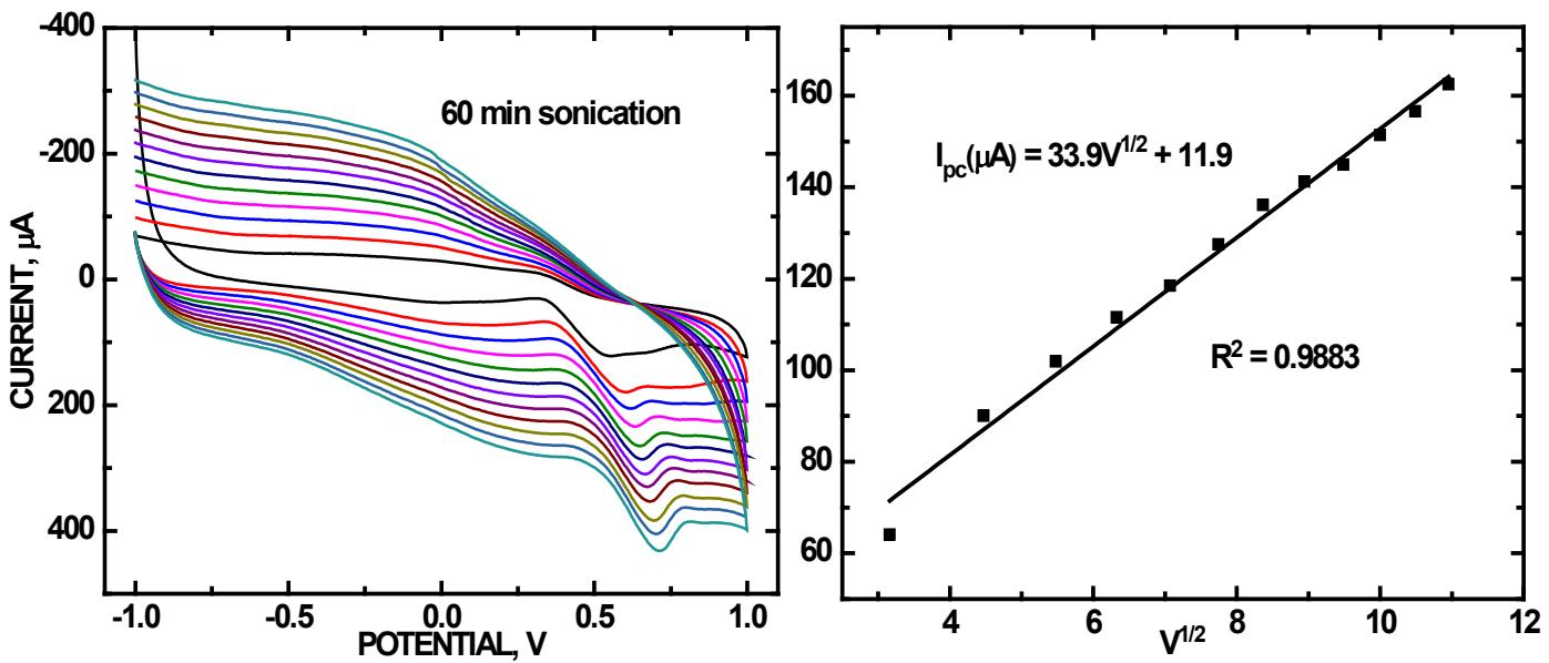
**Figure S2.** CVs of 10 mM UA in PBS (pH = 7.0) at scan rates between 10-100 mV·s<sup>-1</sup> for a 60 min refluxed ZnO/COOH-MWNT composite (left panel). Linear least squares plot from Randles-Sevcik analysis (right panel).
