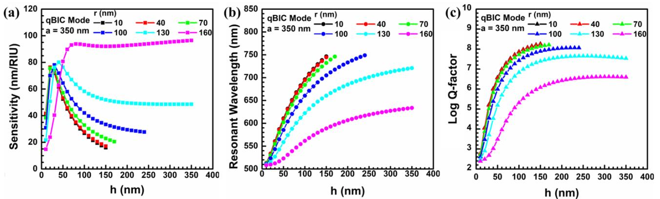
**Figure 7.** The (a) sensitivity, (b) resonant wavelength, and (c) quality factor are determined by different combinations of radii and depths of the nanohole-structured metasurface under the qBIC mode.
