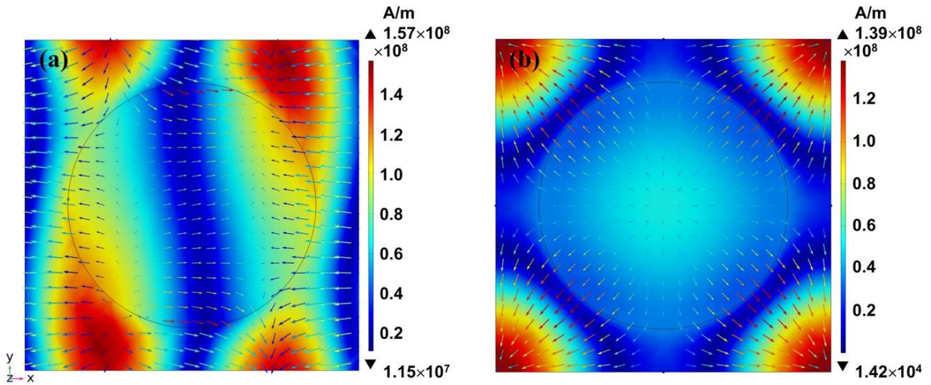
**Figure 6.** The distribution of the magnetic field on the top of the nanohole-structured thin-film layer (e.g., the  $x$ - $y$  plane) in (a) the PR mode and (b) the qBIC mode under the simulation conditions at  $a = 350$  nm,  $r = 130$  nm, and  $h = 40$  nm.
