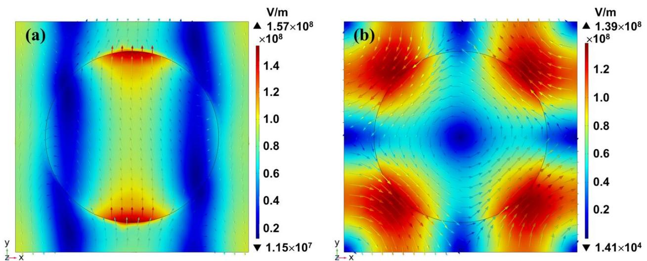
**Figure 5.** The distribution of the electric field on the top of the nanohole-structured thin-film layer (e.g., the x-y plane) in (a) the PR mode and (b) the qBIC mode under the simulation conditions at  $a = 350$  nm,  $r = 130$  nm, and  $h = 40$  nm.
