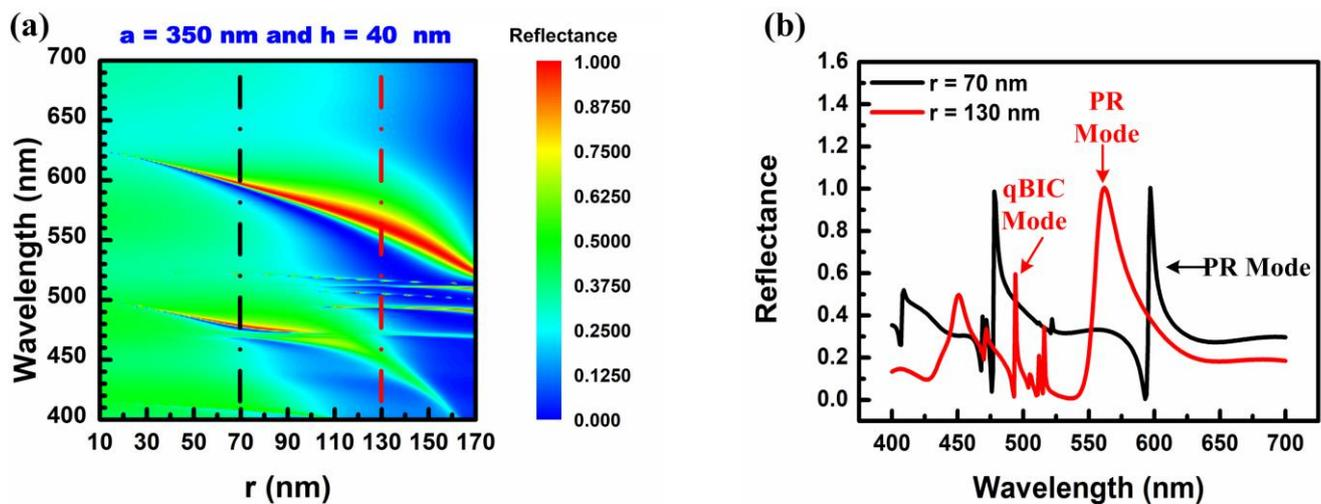
**Figure 3.** (a) The reflectance spectrum of the nanohole all-dielectric metasurface by varying the radius of the nanohole-structured thin-film layer of the all-dielectric metasurface with  $a = 350$  nm and  $h = 40$  nm. (b) The reflectance spectrum of the nanohole-structured thin-film layer of the all-dielectric metasurface with radius ( $r$ ) of 70 nm and 130 nm (black and red dashed line in Figure 3a).
