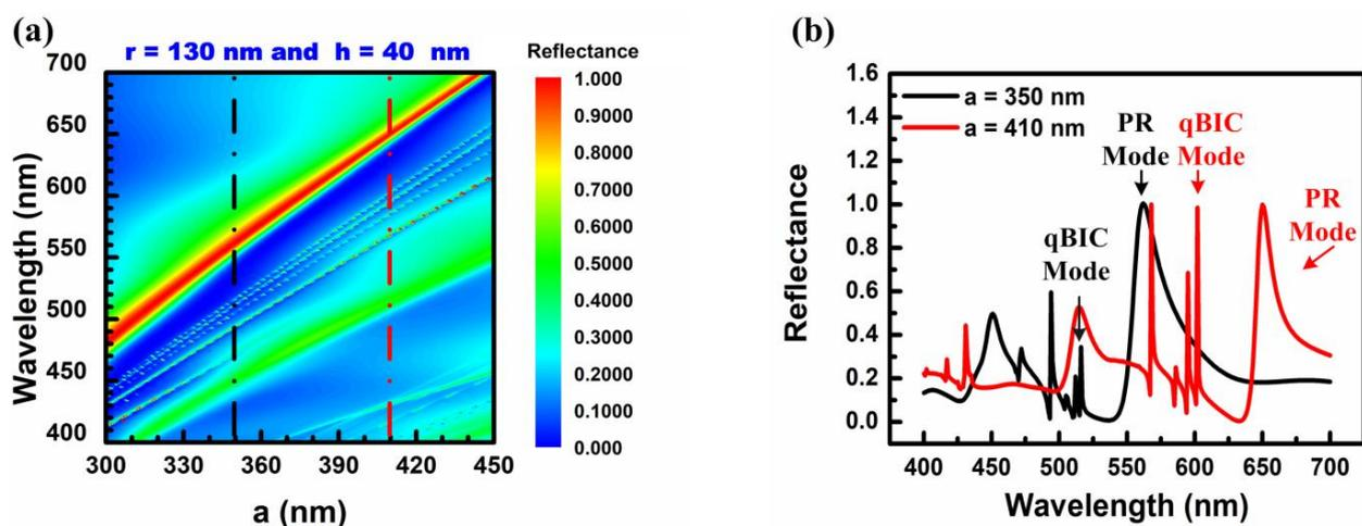
**Figure 2.** (a) The reflectance spectrum of the nanohole all-dielectric metasurface by varying the nanohole-structured thin-film layer's lattice constant of the all-dielectric metasurface with fixed  $r = 130$  nm and  $h = 40$  nm. (b) The reflectance spectrum of the nanohole-structured thin-film layer of the all-dielectric metasurface with lattice constants (a) of 350 and 410 nm (black and red dashed line in Figure 2a). Multiple resonance modes can be found, including the PR and qBIC modes.
