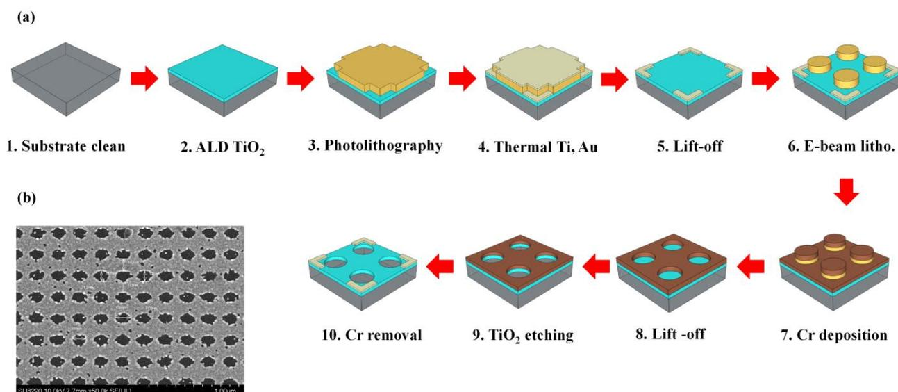
**Figure A1.** (a). The fabrication process of all-dielectric metasurface and (b) scanning electron microscope (SEM) image of the fabricated result of the metasurface.
