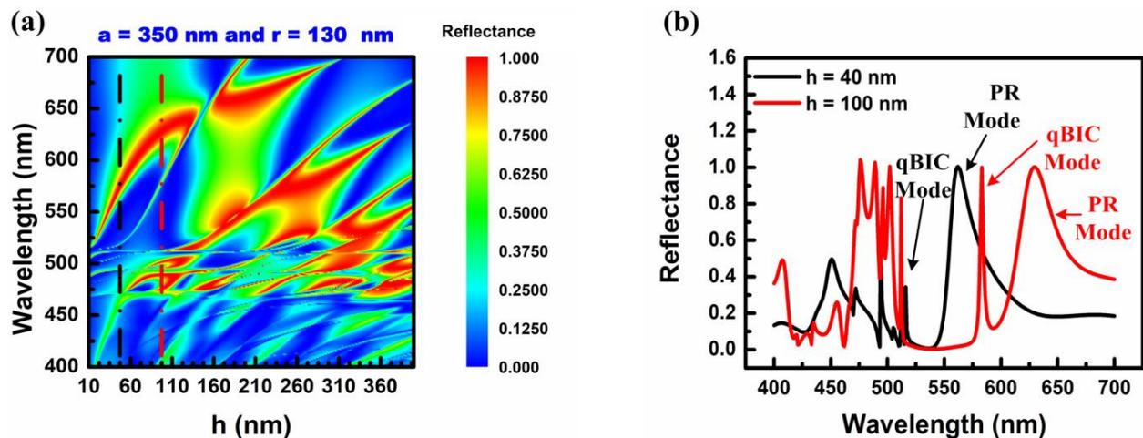
**Figure 4.** (a) The reflectance spectrum of the nanohole all-dielectric metasurface by varying the depth of the nanohole-structured thin-film layer of the all-dielectric metasurface with  $a = 350$  nm and  $h = 40$  nm. (b) The reflectance spectrum of the nanohole-structured thin-film layer of the all-dielectric metasurface with depths ( $h$ ) of 40 and 100 nm (black and red dashed lines in Figure 4a).
