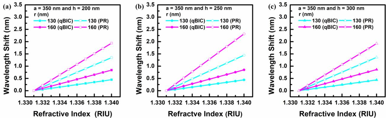
**Figure 9.** The sensor response curves of the proposed all-dielectric metasurface refractive-index sensor operated at the qBIC (solid symbol) mode and the PR mode (open symbol) and radii of the circular hole thin-film structure layer are respectively given as  $r = 130$  nm (light blue-colored symbols) and  $160$  nm (pink-colored symbols), while the depths of the circular hole thin-film structure layer are at (a)  $h = 200$  nm, (b)  $h = 250$  nm, and (c)  $h = 300$  nm.
