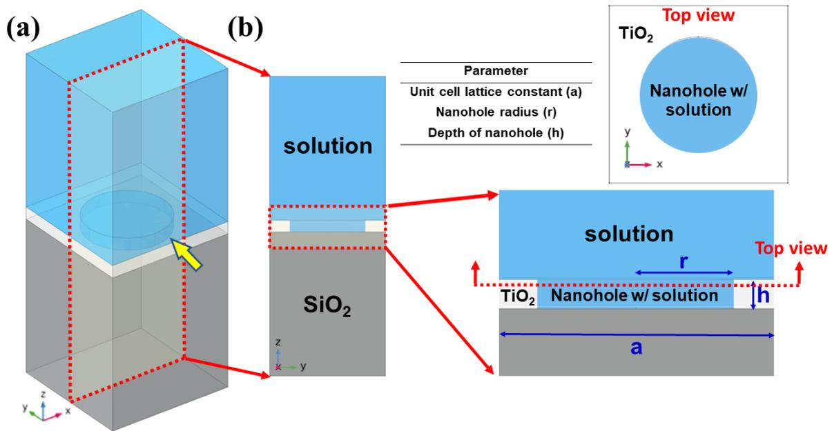
**Figure 1.** (a) Schematic 3D plot and (b) cross-sectional and top views with designed geometric parameters of the designed unit cell of the all-dielectric metasurface composed of a dielectric nanohole-structured thin layer on a solid dielectric substrate.
