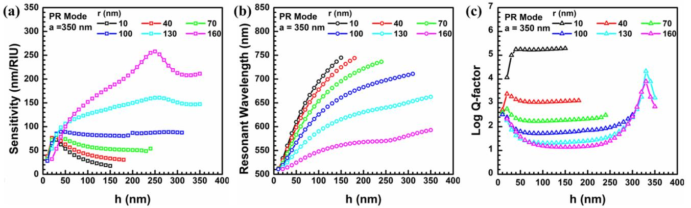
**Figure 8.** The (a) sensitivity, (b) resonant wavelength, and (c) quality factor are determined by different combinations of radius and depth of the nanohole-structured metasurface under the PR mode.
