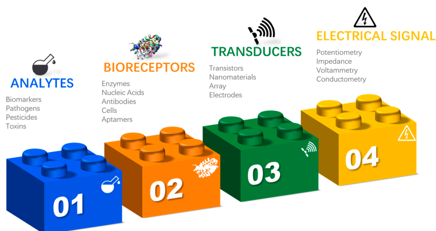
Figure 1. Simplified components' representation of an electrochemical biosensor.
