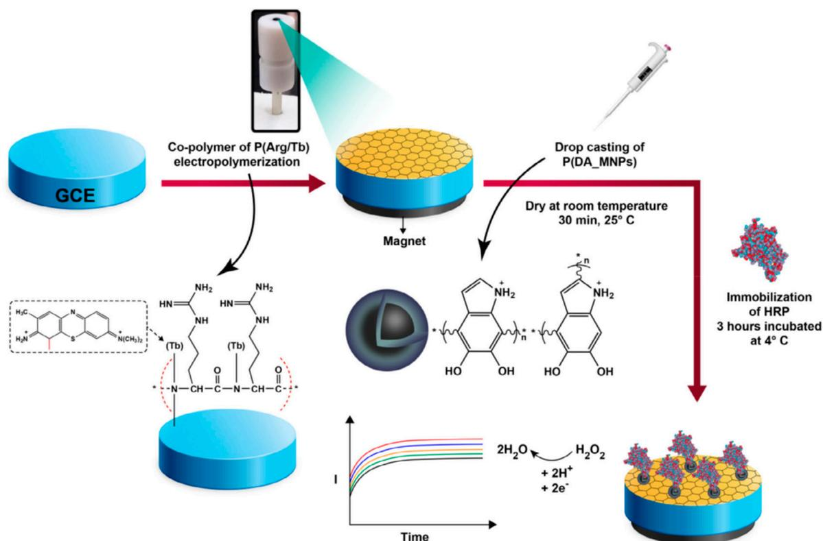
**Figure 5.** Synthesis procedure of HRP/PDA-MNPs/(L-Arg/Tb) hybrid thin film for  $\text{H}_2\text{O}_2$  detection. Taken with permission from Ref. [97]. Copyright 2021. Journal of Molecular recognition.
