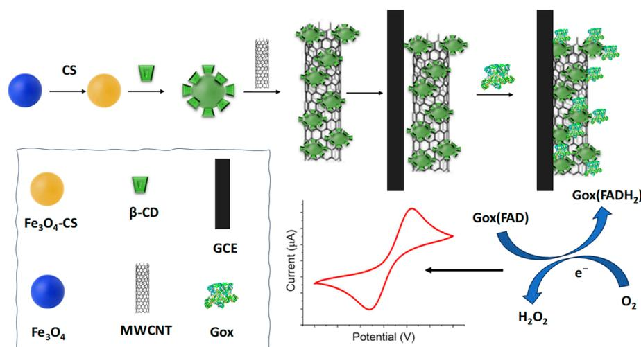
**Figure 2.** Schematic illustration of the fabrication of the glucose biosensor. Reproduced with permission from Ref. [77] Copyright 2020. Electroanalysis.
