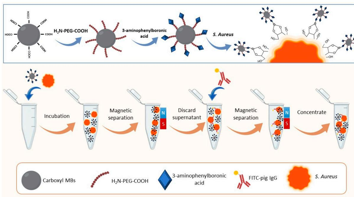
**Figure 3.** Schematic diagram of fluorescence assays combined with APBA-PEG-MNs for *S. aureus* detection. Adapted with permission from Ref. [87]. Copyright 2022. Microchemical Journal.
