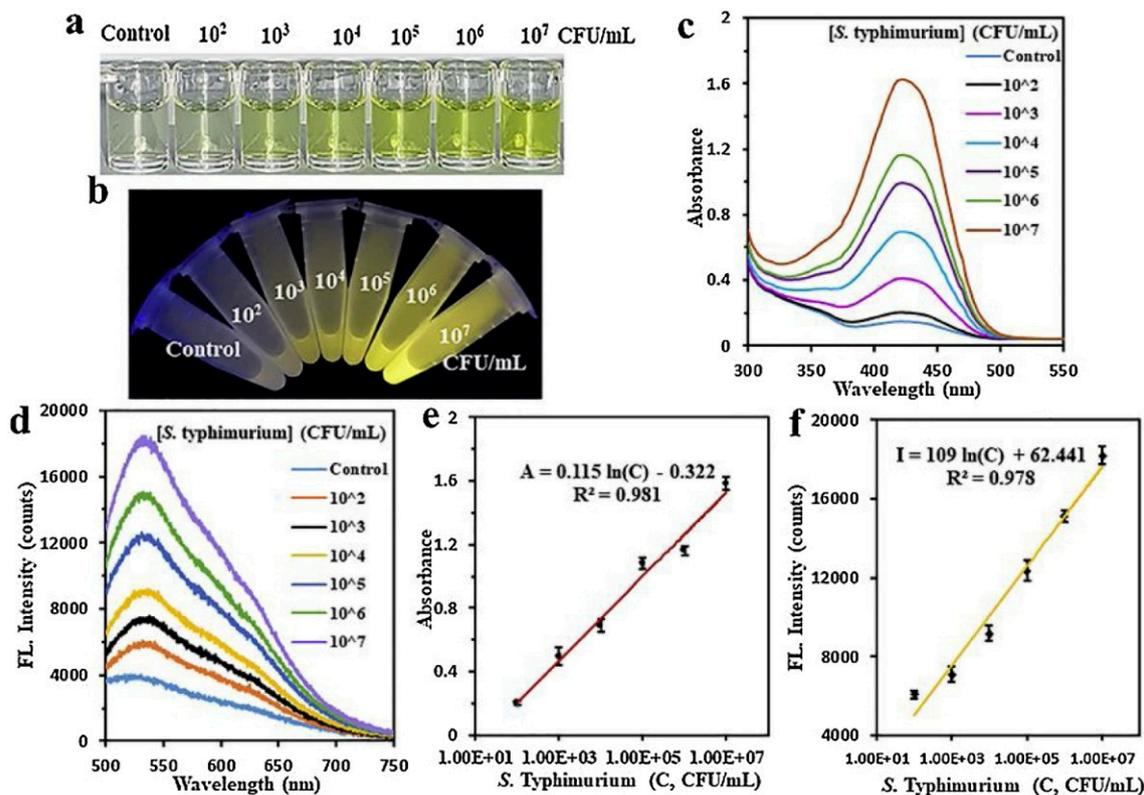
**Figure 6.** Results of ZnO-capped mesoporous silica NPs as a biosensor platform for *S. Typhimurium* detection: (a) absorbance and (b) fluorescence photographs; (c) absorbance and (d) fluorescence spectra; calibration curve of (e) absorbance and (f) fluorescence intensity. Taken with permission from Ref. [99]. Copyright 2020. Sensors and Actuators B: Chemical.
