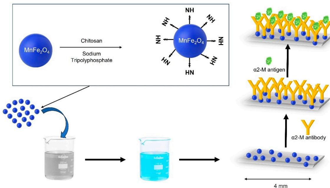
**Figure 1.** Schematic diagram for the synthesis of the MnFe<sub>2</sub>O<sub>4</sub>@chitosan/MWCNTs/PDMS composite film and its integration in an α2 m sensing platform. Adapted with permission from Ref. [56]. Copyright 2023. Creative Commons license.
