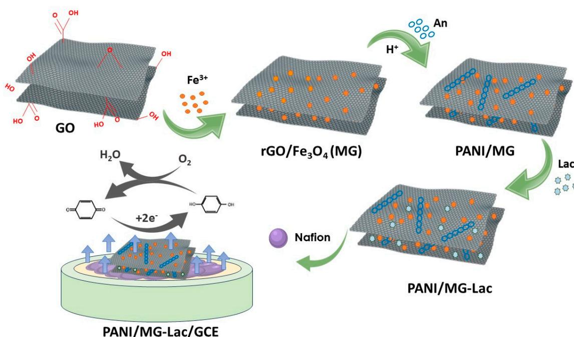
**Figure 4.** Schematic illustration of the synthesis of polyaniline/magnetic graphene-Lac-GCE, along with the enzymatic oxidation of hydroquinone using laccase and its subsequent electrochemical reduction on the GCE. Adapted with permission from Ref. [93]. Copyright 2020. Int J Biol Macromol.
