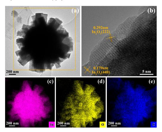
**Figure 4.** (a) TEM image, (b) high-resolution TEM image, and (c-e) its corresponding elemental mapping of 5-rGO/In<sub>2</sub>O<sub>3</sub> composites.
