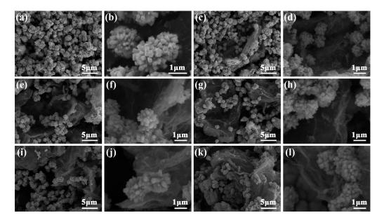
**Figure 3.** FE-SEM images of (**a**,**b**) In<sub>2</sub>O<sub>3</sub>, (**c**,**d**) 1-rGO/In<sub>2</sub>O<sub>3</sub>, (**e**,**f**) 3-rGO/In<sub>2</sub>O<sub>3</sub>, (**g**,**h**) 5-rGO/In<sub>2</sub>O<sub>3</sub>, (**i**,**j**) 7-rGO/In<sub>2</sub>O<sub>3</sub>, and (**k**,**l**) 10-rGO/In<sub>2</sub>O<sub>3</sub>.
