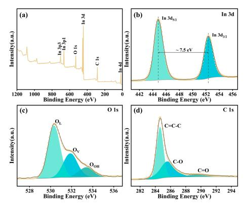
**Figure 5.** (a) Survey XPS spectra of 5-rGO/In<sub>2</sub>O<sub>3</sub>, (b) XPS spectrum of In, (c) XPS spectrum of O, and (d) XPS spectrum of C.
