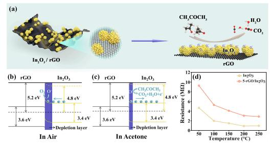
**Figure 9.** (a) Schematic diagram of the mechanism of the acetone gas-sensing process of the  $rGO/In_2O_3$  composites. (b,c) Schematics of energy band diagrams of  $rGO/In_2O_3$  heterojunctions. (d) The resistance of the sensors in air as a function of operating temperature.
