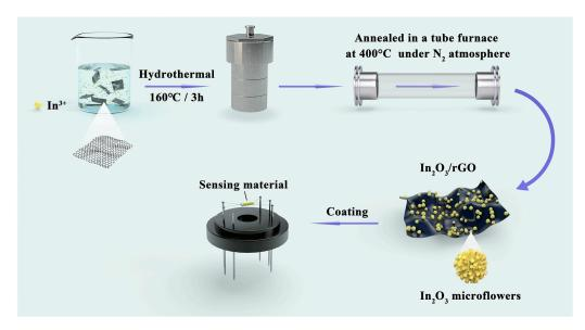
Figure 1. The schematic of the synthesis process of the rGO/In<sub>2</sub>O<sub>3</sub> composites.
