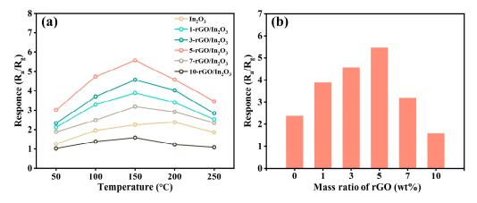
**Figure 7.** (a) The sensing response to 10 ppm acetone at various operating temperatures. (b) Correlations between the sensing response to 10 ppm acetone at the optimal operating temperature and rGO mass ratios.
