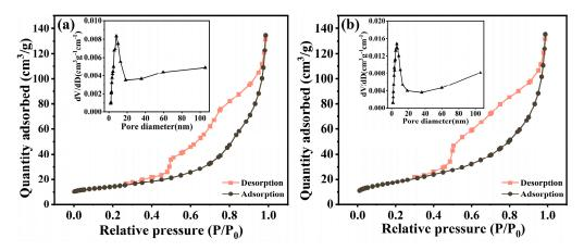
**Figure 6.** Typical N<sub>2</sub> adsorption–desorption isotherm and pore size distribution plots (inset) of (a)  $In_2O_3$  and (b) 5-rGO/In<sub>2</sub>O<sub>3</sub>.
