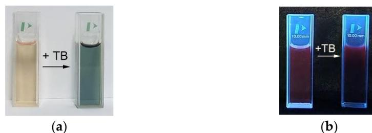
**Figure 7.** Photographic images of the Pt-allyloxy-TSPP trimer before and after exposure to TB, (a) in visible light and (b) under ultraviolet irradiation at 254 nm.
