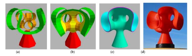
**Figure 11.** *The Lighthouse*: (**a**) the key features; (**b**) 1/3 of the control surface is added; (**c**) model after smoothing and offsetting; and (**d**) the resulting 3D printed object.
