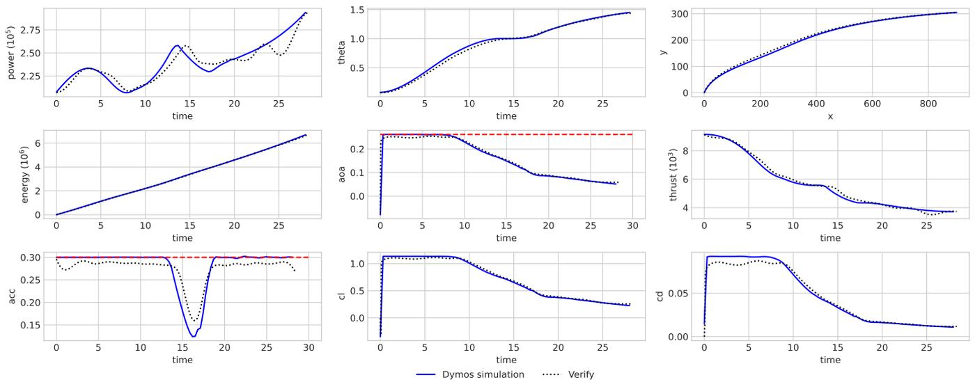
**Figure 5.** We verified results with Dymos package. The blue line represents the direct result of the outputs from the Dymos optimization data by NASA, and the black dot line presents the results by Chauhan and Martins [14] as verification data. The units for each y axis are given by the following: power (W), theta (rad), y (m), energy (J), aoa (rad), thrust (N), acc (g), cl (-), cd (-).
