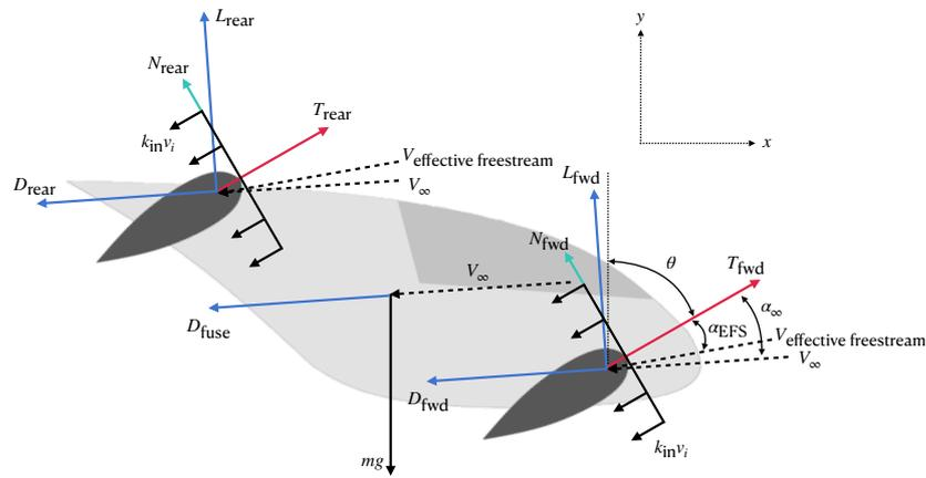
**Figure 1.** Definitions of angle and forces on the aircraft.
