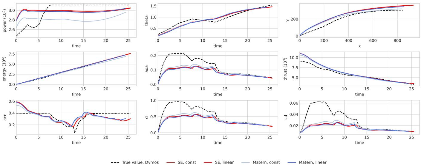
**Figure 6.** Optimized takeoff trajectory profile for MOGP models 1–4 verified against simulation-based ground truth.
