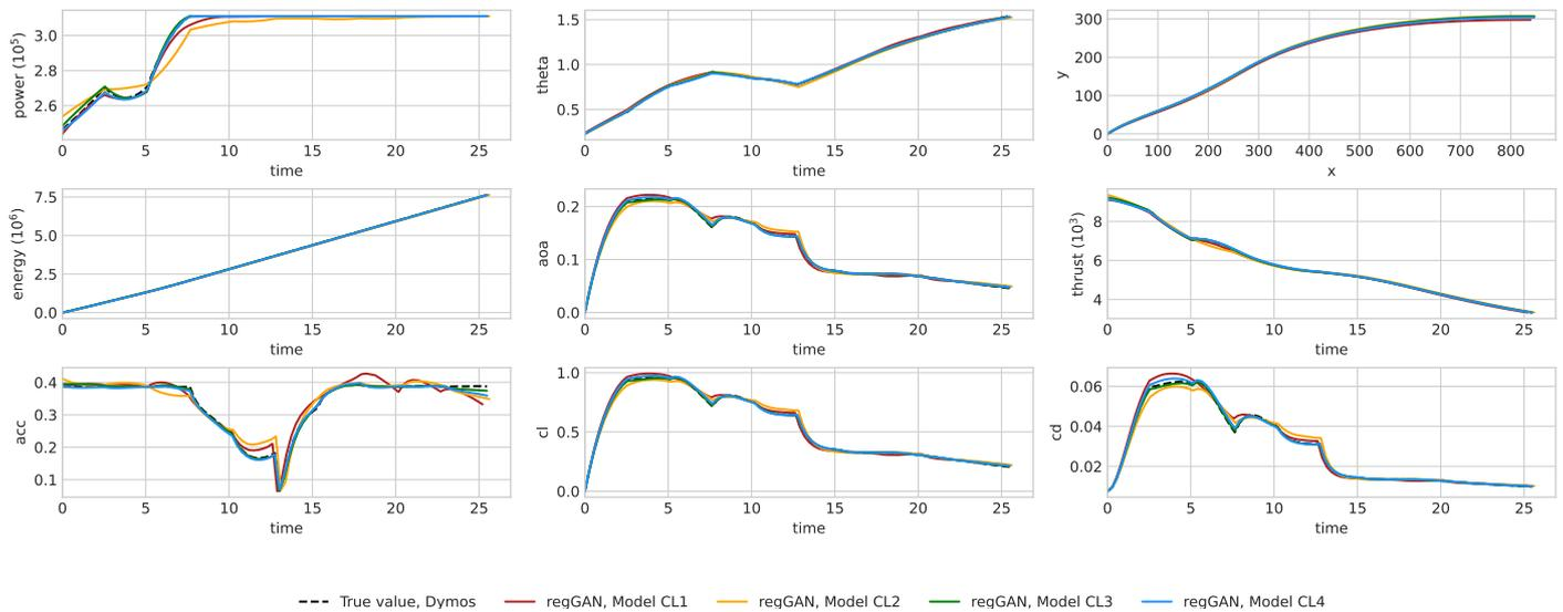
**Figure 9.** Optimal takeoff trajectory profiles predicted by regGAN models CL1–4 match well with simulation-based ground truth.
