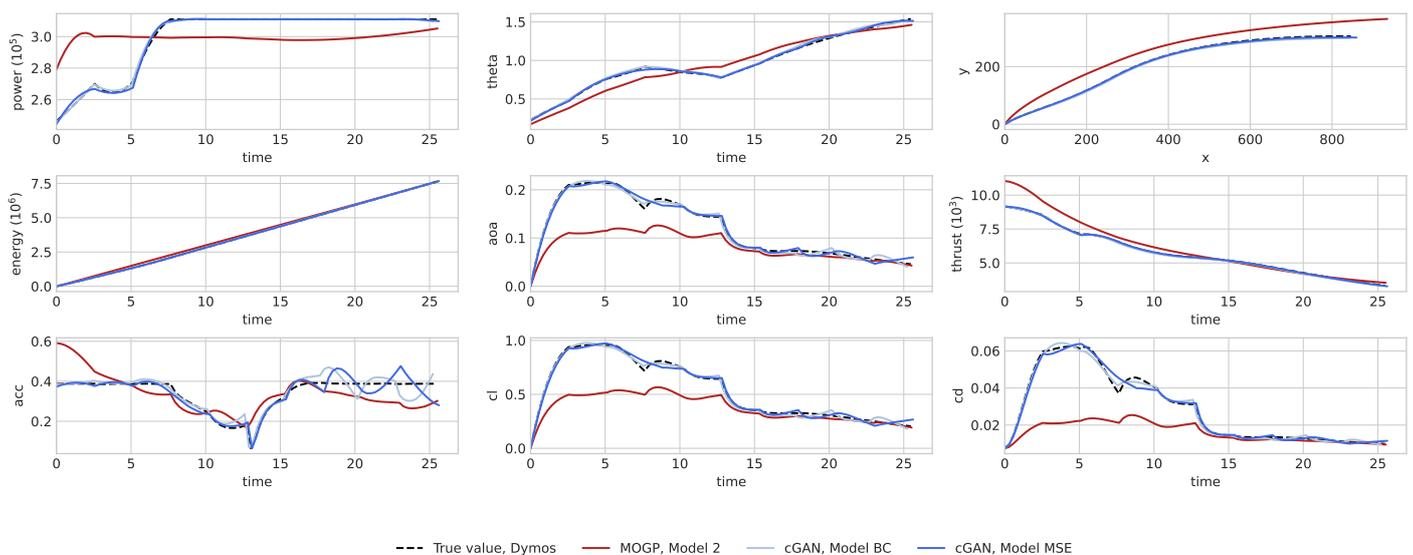
**Figure 7.** Optimal takeoff trajectory profile comparison on cGAN model BC and MSE and MOGP model 2 with simulation-based ground truth.
