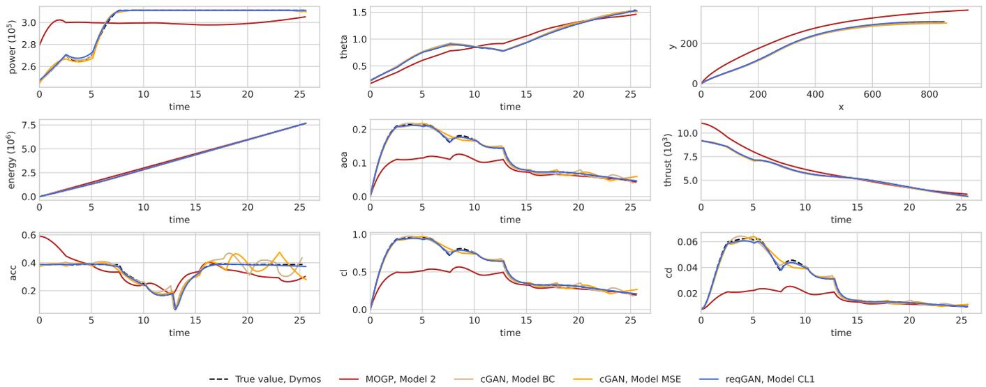
**Figure 8.** Optimal takeoff trajectory profile for regGAN model CL1 matches the ground truth and outperforms cGAN models BC and MSE and MOGP model 2.
