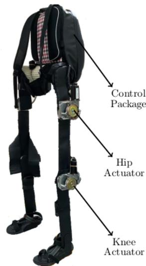
Figure 1. Structure of the wearable lower-limb exoskeleton.
