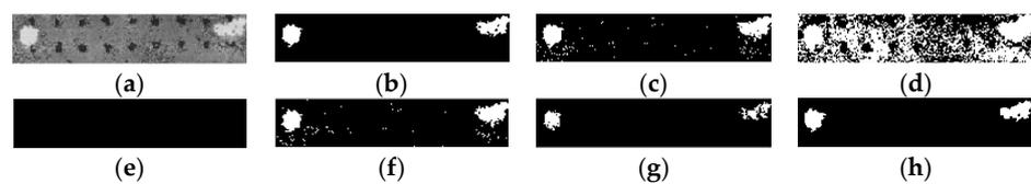
**Figure 9.** Image13 and its segmentation results: (a) #image13, (b) ground-truth, (c) Otus, (d) MRCUT, (e) EITMIS, (f) NSWCC, (g) IT2FSWCC, (h) FSEFTISRI.
