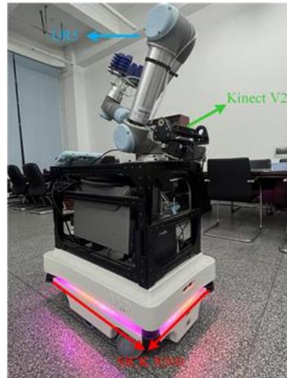
**Figure 12.** Mobile robot platform. The platform is equipped with a Kinect V2 sensor for visual inspection, a UR5 robotic arm for object grasping and two SICK S300 LIDARs on the chassis that can be used to acquire point cloud information about the surrounding environment for navigation research.
