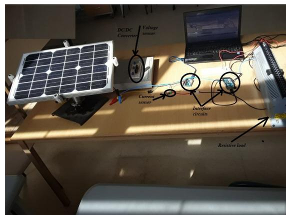
Figure 13. The proposed photovoltaic circuit.
