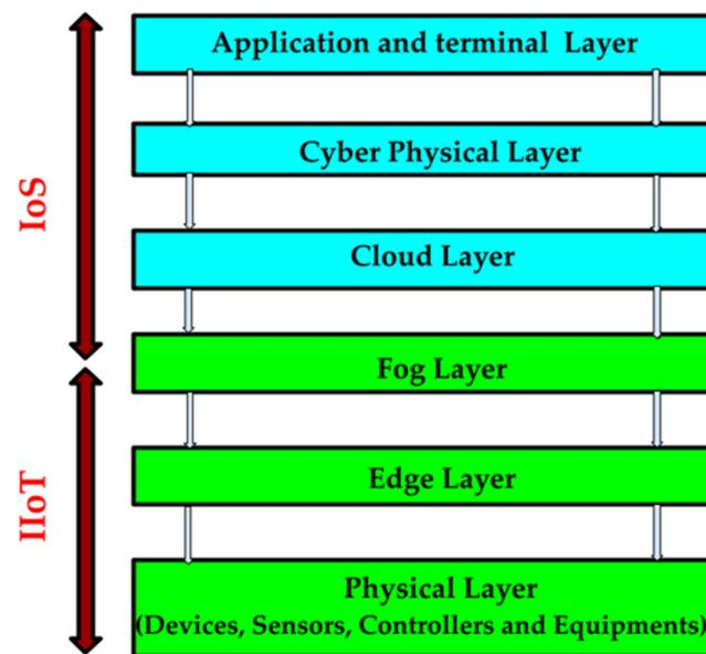
**Figure 2.** Interface between Internet of Services (IoS) and Industrial IoT (IIoT), and its interface with network architecture for the smart factory.
