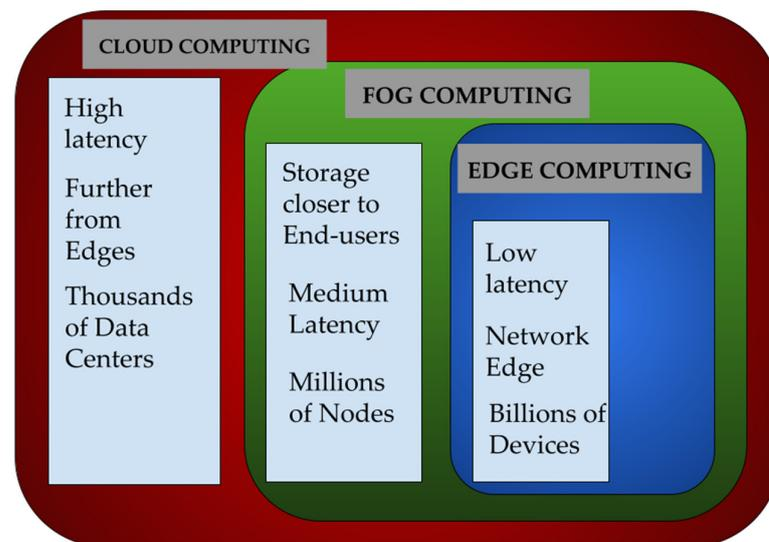
**Figure 6.** Hierarchical architecture and structural relationship between Cloud, Fog, and Edge computing.
