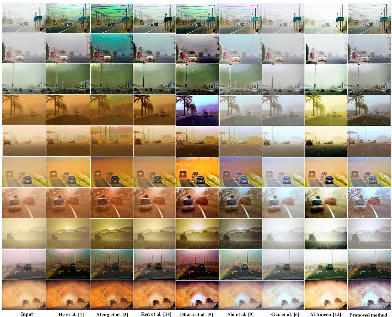
**Figure 8.** The comparison of existing dehazing methods and the proposed method.
